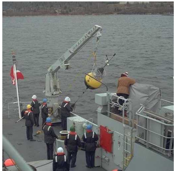
Figure 1: Launching of Wave Buoy from Side of Ship Using a Boom Crane
