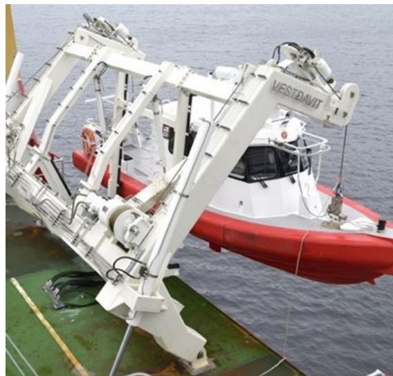
Figure 4: Boat Attached to Davit with Dual Lift Points (courtesy of Vestdavit)
