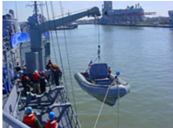
Figure 2: Boat Attached to Crane with Single Lift Hook (courtesy of Welin Lambie)
