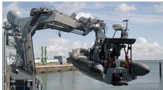
Figure 3: Boat Attached to Davit with Rigid Lift Connection (courtesy of Vestdavit)
