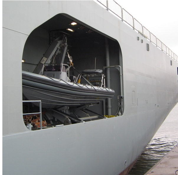
Figure 5: Boat Launch and Recovery System Inside Alcove on Ship (courtesy of Vestdavit)
