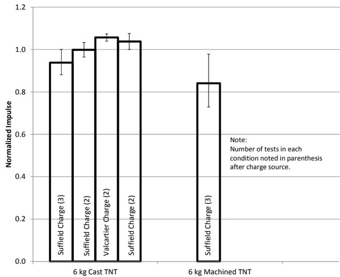
Figure 4: Comparison of normalized impulse for cast and machined 6 kg TNT charges.
