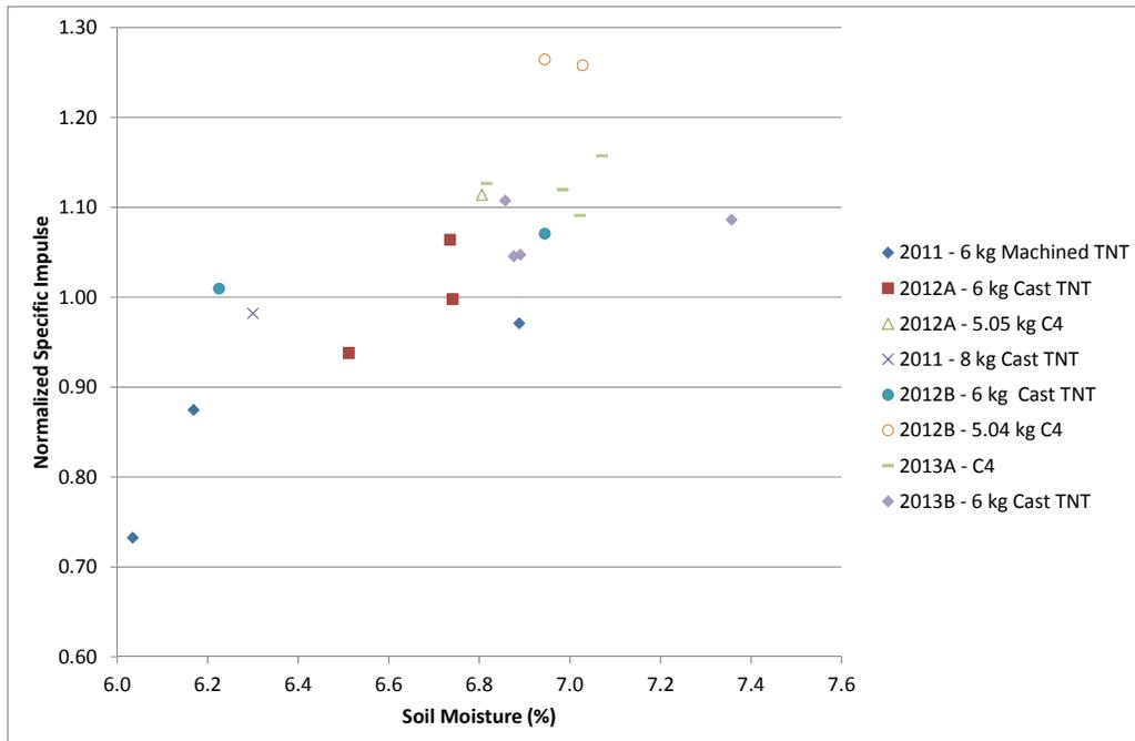
Figure 6: Effect of soil pit moisture content on normalized specific impulse.
