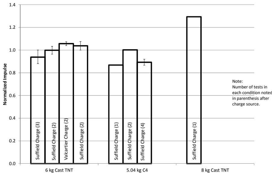
Figure 5: Comparison of normalized impulse for C4 and cast TNT charges.
