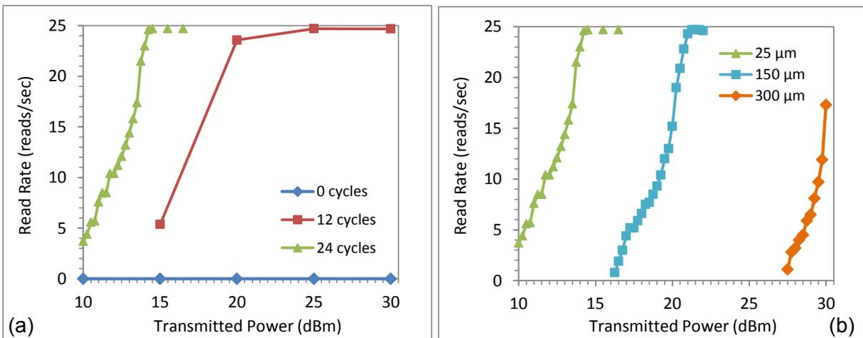
**Figure 3: Read rate vs. transmitted power for RFID tags coated with steel shim stock and subjected to accelerated corrosion cycles (a) 25  $\mu\text{m}$  shim stock following 0, 12 and 24 corrosion cycles (b) 25, 150 and 300  $\mu\text{m}$  shim stock following 24 corrosion cycles**
