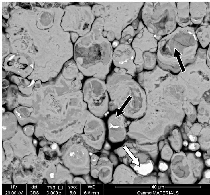
**Figure 5: SEM image of cross section of composite coating after 24 corrosion cycles. The uncorroded steel particles appear as white regions (white arrow) while the oxides appear as darker grey regions (black arrows).**
