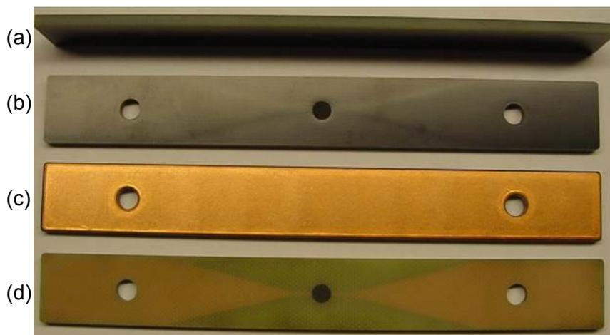
**Figure 1: RFID tags, showing (a) edge profile, (b) top surface of tag, (c) bottom surface of tag with built-in metal backplane, and (d) top surface of tag with plastic casing removed.**
