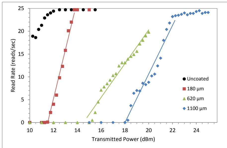
**Figure 2: Read rate vs. transmitted power for RFID tags coated with 0, 180, 620, 1100 μm thick 75 wt% steel/acrylic resin composite coatings. (0 corrosion cycles, linear trend-lines added for emphasis)**
