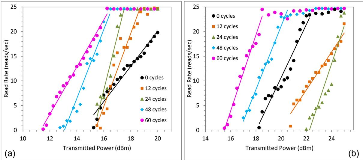
**Figure 4: Read rate vs. transmitted power for RFID tags with (a) 620 μm and (b) 1100 μm thick composite coatings following 0, 12, 24, 48, and 60 corrosion cycles. Linear trend lines added for emphasis.**
