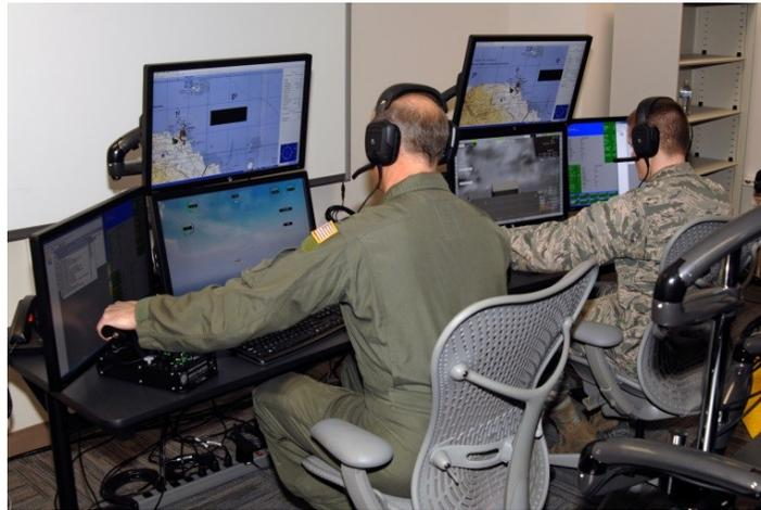
**Figure 1. TIGER Air Vehicle Operator and Sensor Operator workstations**
