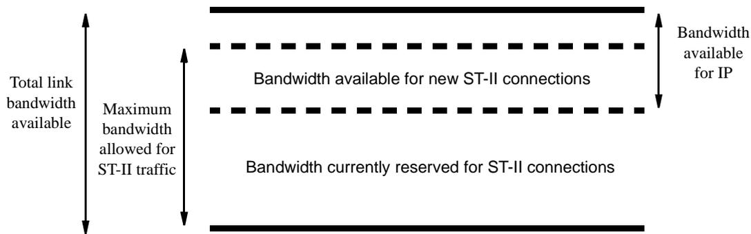
**Figure 26.** IP and ST-II bandwidth allocation
