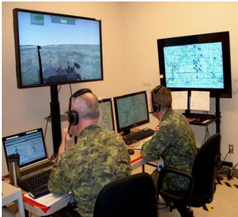
*Figure 1:* Command on the move Tactical Command Post. The Unit Commander sits to the right having the planning and COP monitors in front of him. The battle adjutant staffs the computer with chat, email, and file sharing capabilities and assists the Unit Commander with the planning functions.
