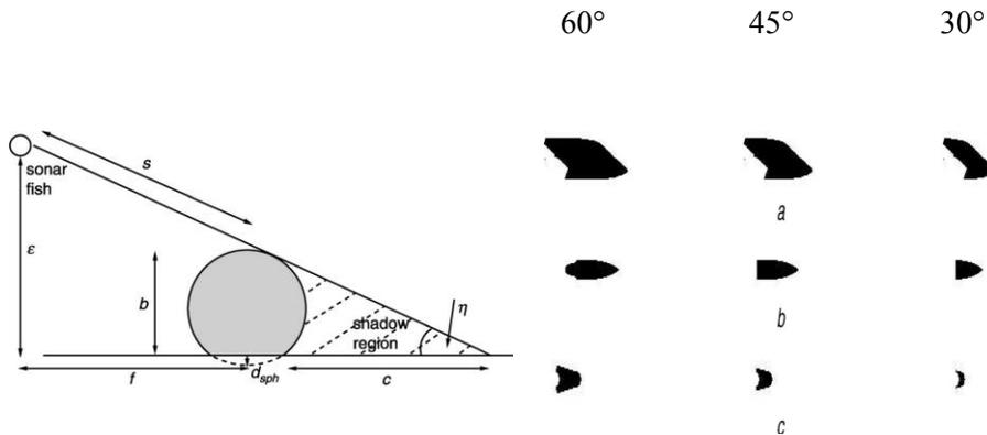
Figure 5: The shadow regions under different incident angles [7]
