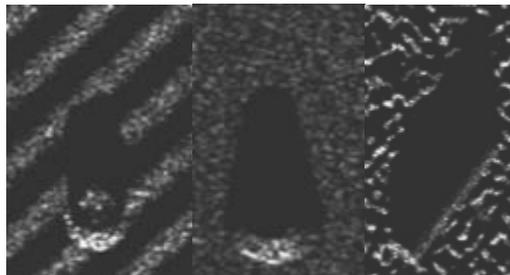
Figure 3: Sonar images of targets in different sea-beds [5]
