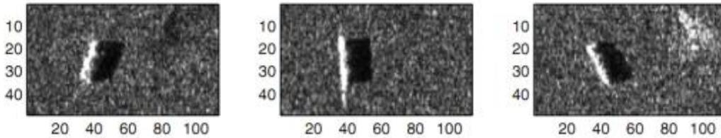
Figure 4: Sonar images in pixel of a cylinder at different aspect angles ( $30^\circ$  increments) [6]
