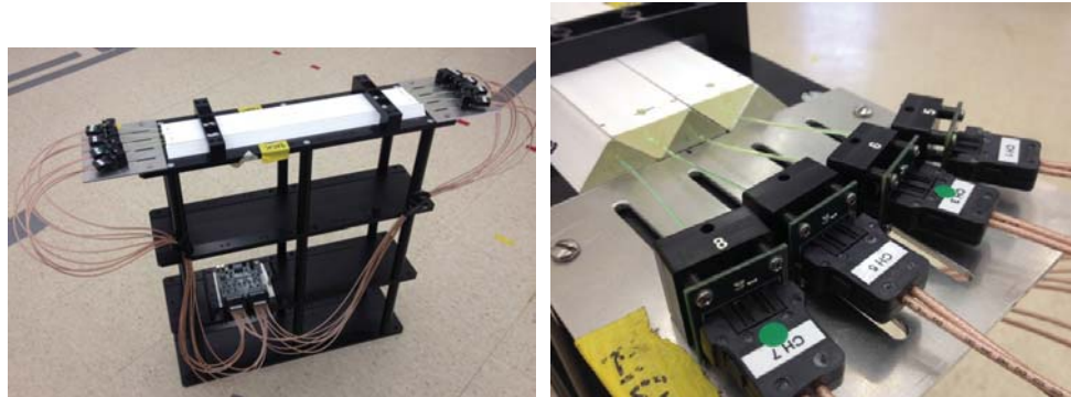
Figure 2.1: Four 45-cm long triangular plastic scintillator bars with Kuraray Y-11 1.2 mm diameter WLS fibres along their centres. Both ends of each fibre were connected to Hamamatsu S12572-050C SiPMs connected to a Vertilon SIB-108 board and a Vertilon IQSP482 charge integrating DAQ.
