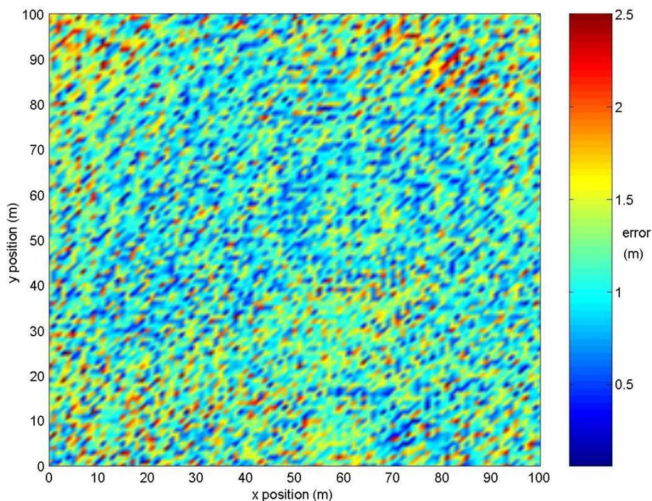
**Figure 5.** Accuracy of a TOA system with a chip rate of 122.88 Mcps
