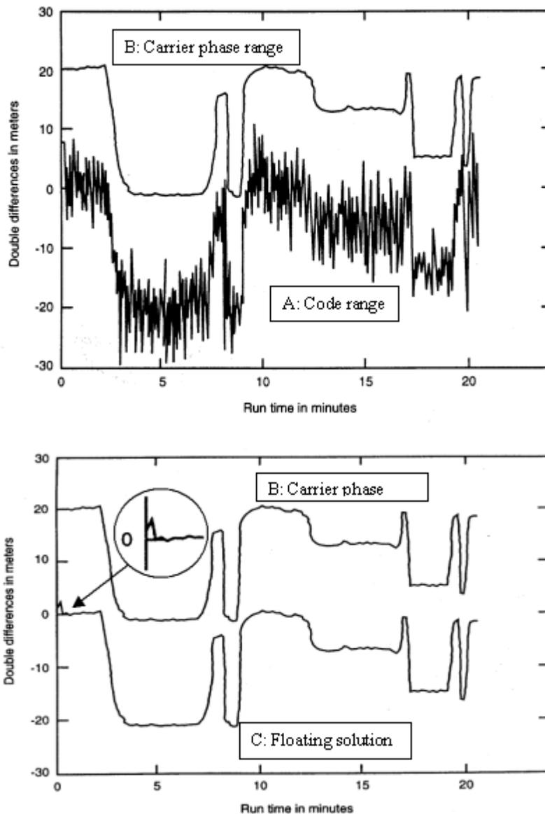
**Figure 2. The floating solution C derived from the code range A and the carrier phase range B by a Kalman filter (from 2, p366-367).**
