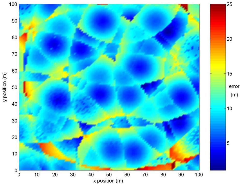
**Figure 4.** Accuracy of a TOA system with a chip rate of 1.2288 Mcps.
