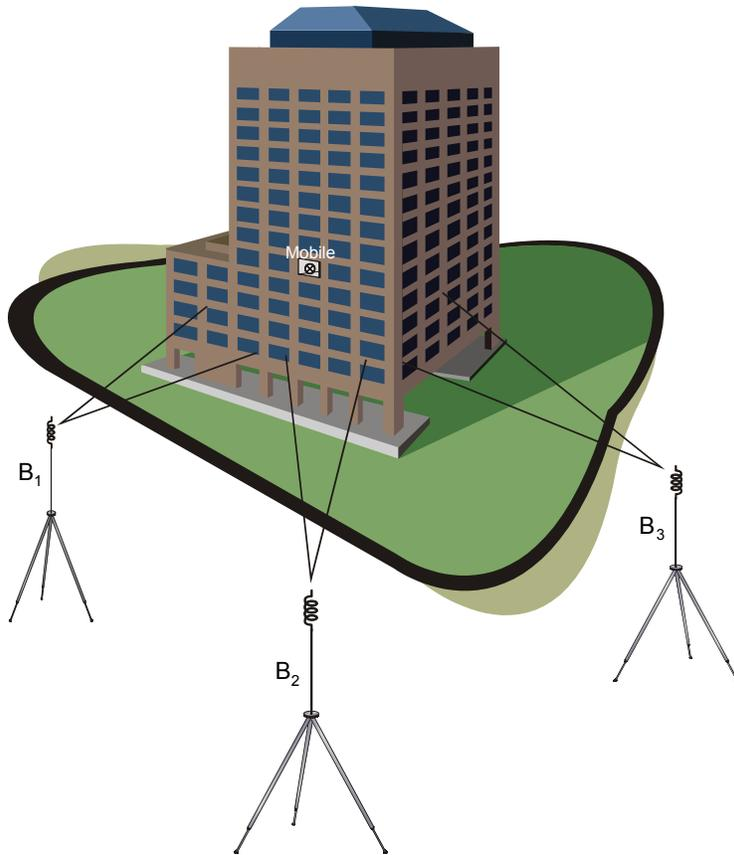
**Figure 3. Proposed architecture for indoor geolocation.**
