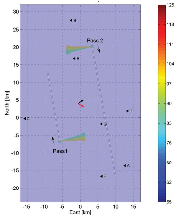
Fig. 1. Flight geometries in the East-North-Up coordinate system. Wind direction and swell direction are indicated by the black and the red arrows, respectively. The color codes the steering direction [°] of the antenna.
