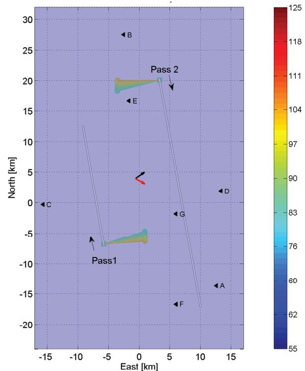
Fig. 1. Flight geometries in the East-North-Up coordinate system. Wind direction and swell direction are indicated by the black and the red arrows, respectively. The color codes the steering direction [ $^\circ$ ] of the antenna.
