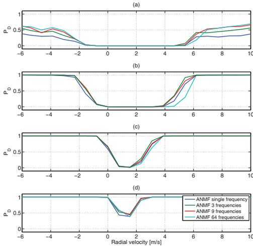
Fig. 3. Probability of detection for  $P_{FA}=10^{-4}$ . SNR range is (a) 7 dB, (b) 13 dB, (c) 25 dB and (d) 31 dB.
