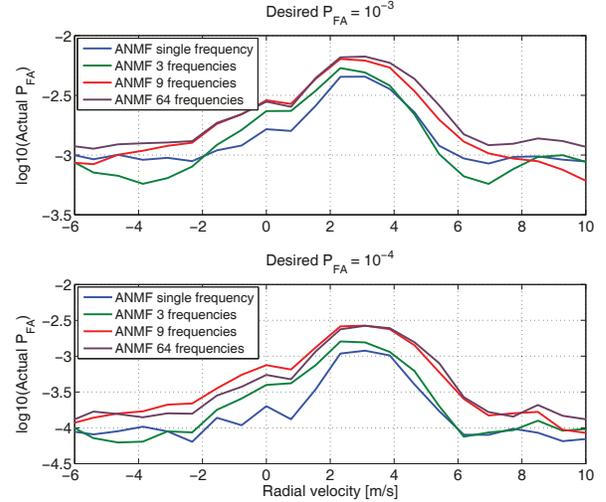
Fig. 2. Actual PFA achieved versus Doppler velocity for ANMF detection with  $\mathbf{z}_f^\dagger \mathbf{M}_f^{-1} \mathbf{z}_f$  summation lengths of 1, 3, 9 and 64 frequency bins. Threshold set to achieve  $P_{FA}=10^{-3}$  and  $P_{FA}=10^{-4}$  for SIRP clutter statistics. Upwind viewing geometry.
