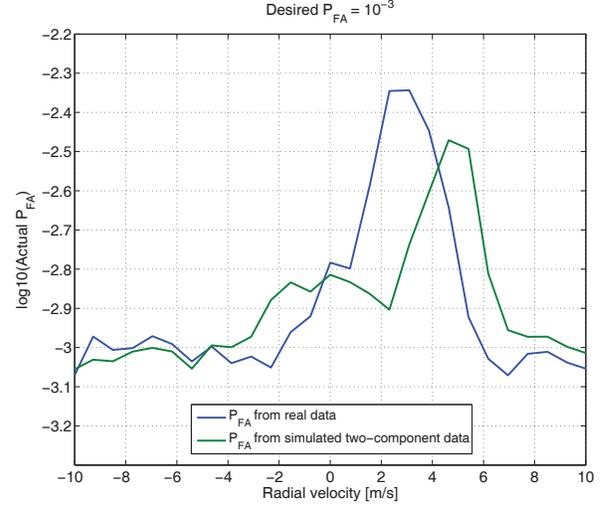
Fig. 4. Measured PFA output from ANMF detector with threshold set to achieve  $P_{FA}=10^{-3}$ . Blue curve corresponds to performance against real PAMIR data. Green curve corresponds to performance against simulated data using equation (13).
