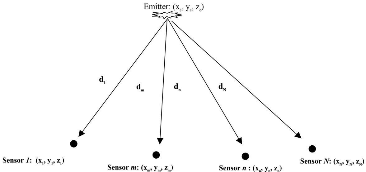
**Figure 1.** Location based on TDOA method using multiple stationary sensors
