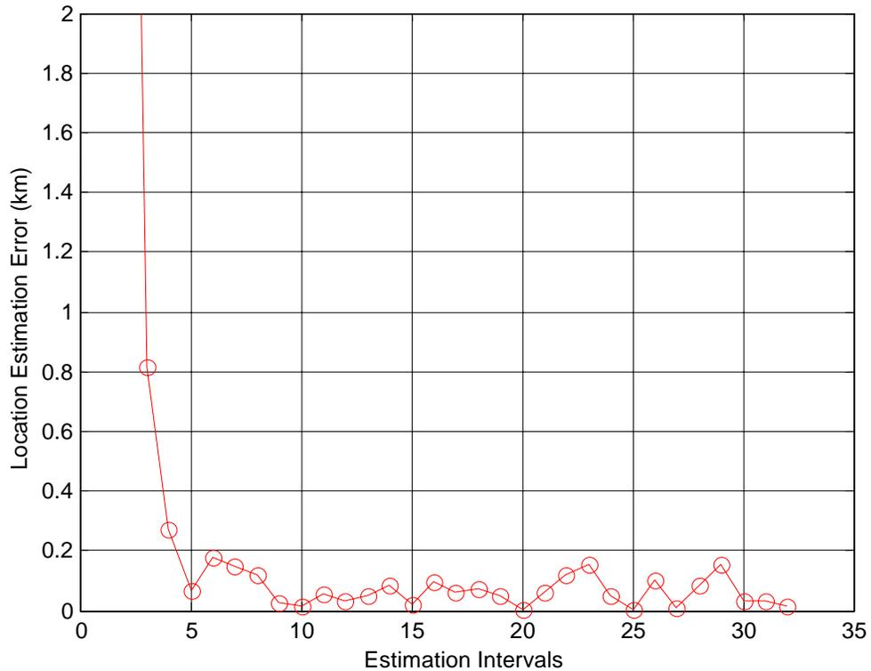
**Figure 6.** Location estimation errors with random TDOA measurement noise
