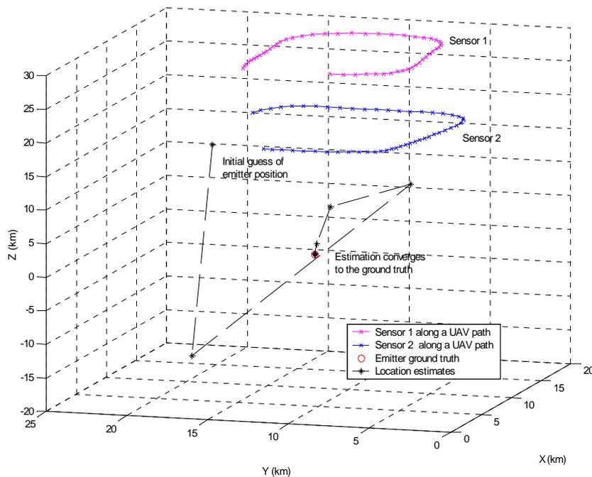
**Figure 9.** Location estimation against the ground truth with random and non-random TDOA measurements noises
