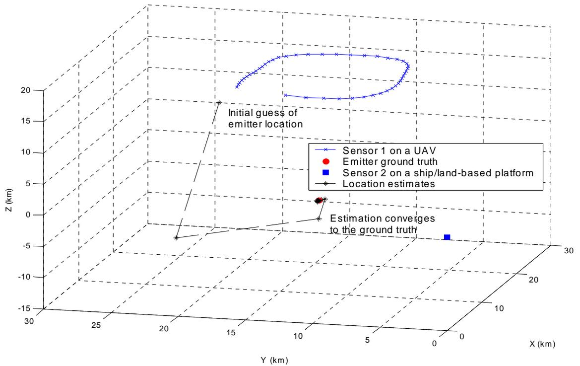
**Figure 5.** Location estimation against the ground truth with random TDOA measurement noise
