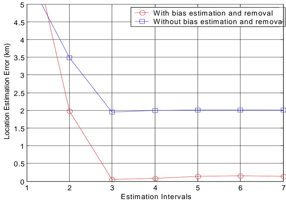
**Figure 8.** Location estimation errors with random and non-random TDOA measurement noises
