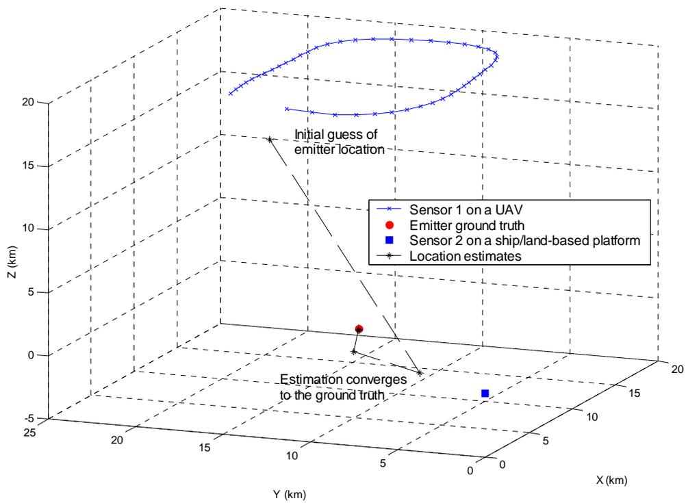
**Figure 7.** Location estimations against the ground truth with random and non-random TDOA measurements noises
