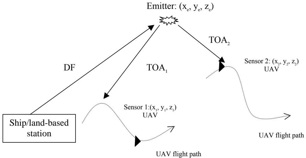
**Figure 3.** Location using TDOAs from two UAVs and a ship/land-based platform
