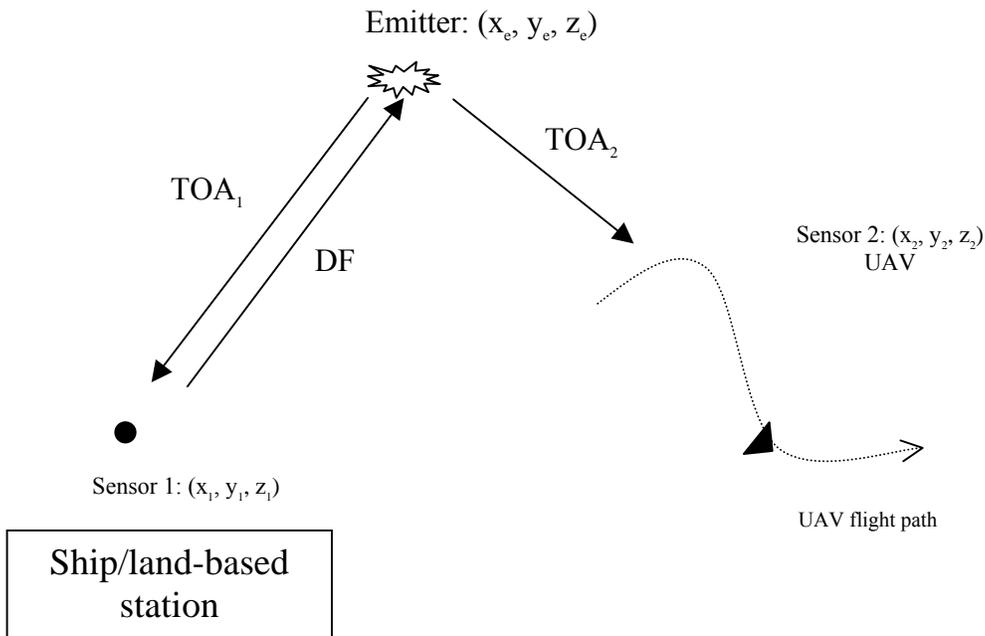
**Figure 2.** Location using TDOAs from a UAV and a ship/land-based platform
