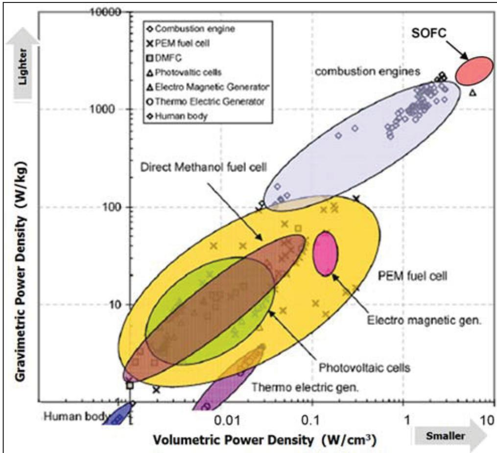
Legend: proton exchange membrane (PEM) fuel cell; and solid oxide fuel cell (SOFC).
