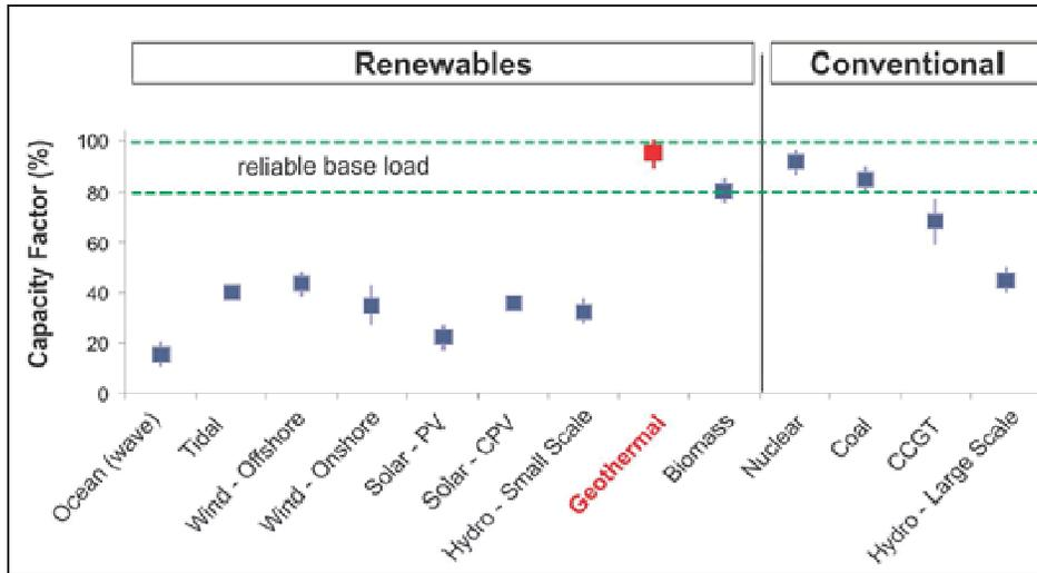
PV = photovoltaics; CPV = concentrated photovoltaics; CCGT = combined-cycle gas turbine.
