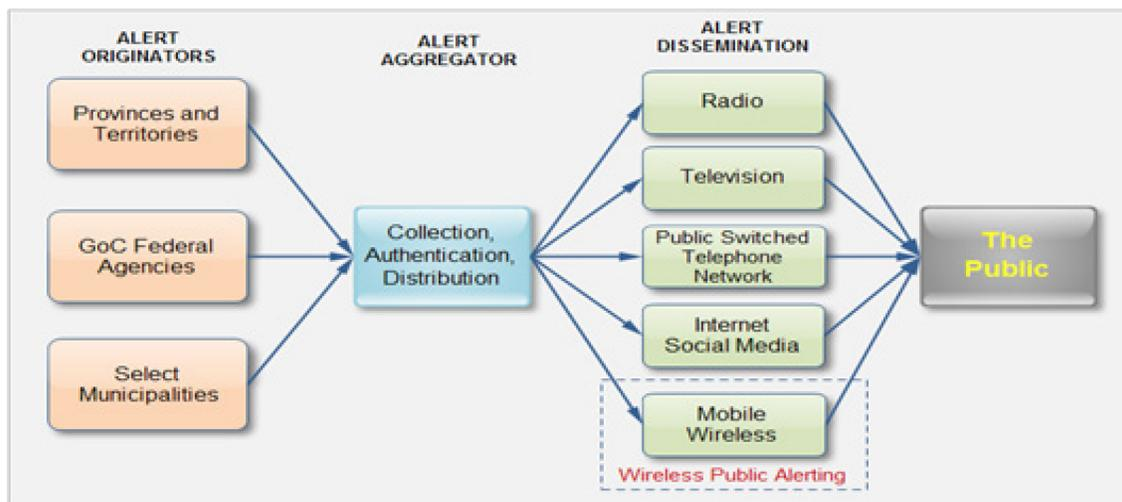
**Figure 1:** Illustration of the flow of alert messages envisioned for a Canadian Public Alerting System (source: Ref. 1).
