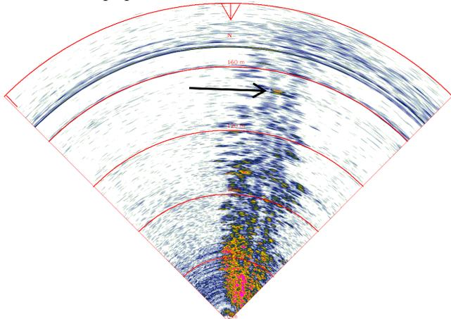
**Figure 2:** Aft-looking HF sonar image to 200 m range, 1128h April 13<sup>th</sup> in Saanich Inlet. Range rings are 40 m increments. Arrow denotes location of towed target.
