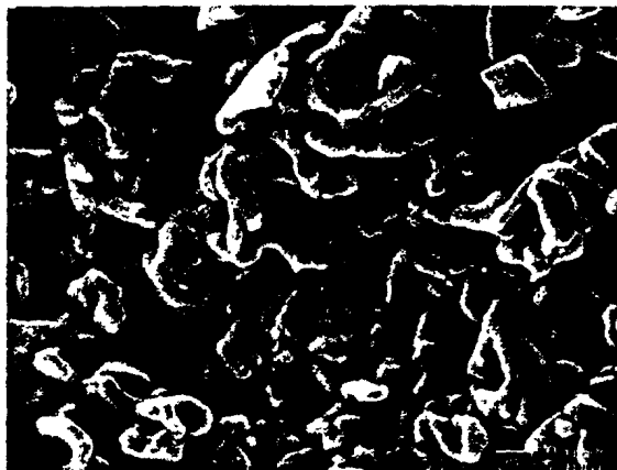
Figure 5a: Scanning electron micrograph of the dense growth of MWNT obtained from ethylene at 700°C on NiCo catalyst in silicate covered carbon fibers
