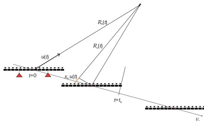
**Figure 2:** Range and direction time history of a moving antenna array.
