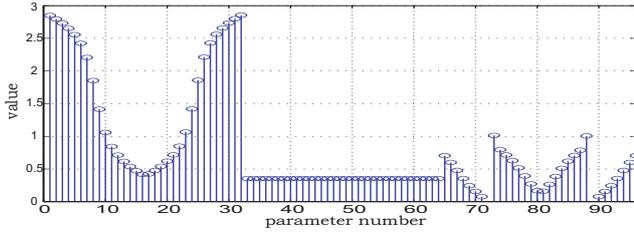
**Figure 3:** Optimum antenna tapering settings.
