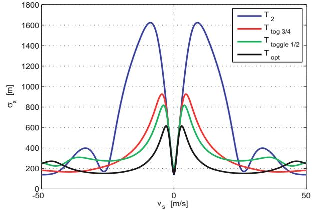
**Figure 6:** CRB for azimuth position at  $v_x = 0$ .
