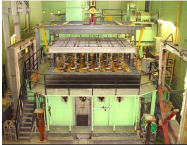
Figure 3. NRC full-scale floor furnace for testing slabs/beams.
