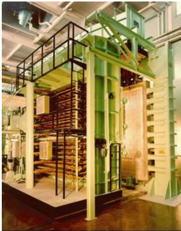
Figure 2. NRC full-scale wall furnace for testing load and non-loaded walls.
