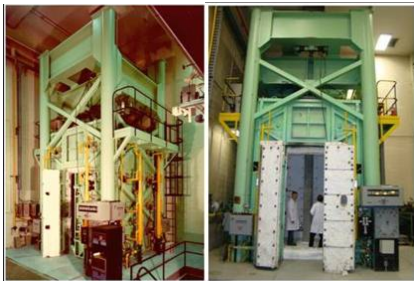
Figure 16. NRC's Column Furnace Facility.
