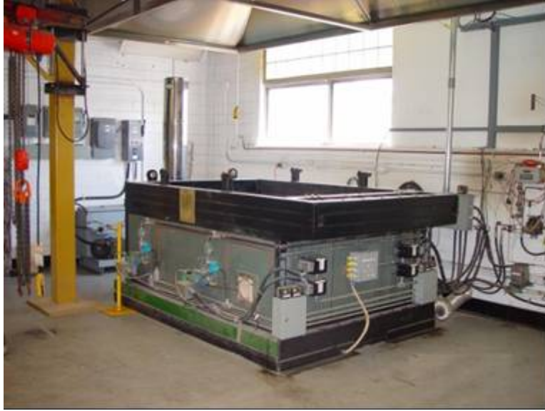
Figure 5. NRC intermediate-scale furnace for testing walls/floors/slabs.
