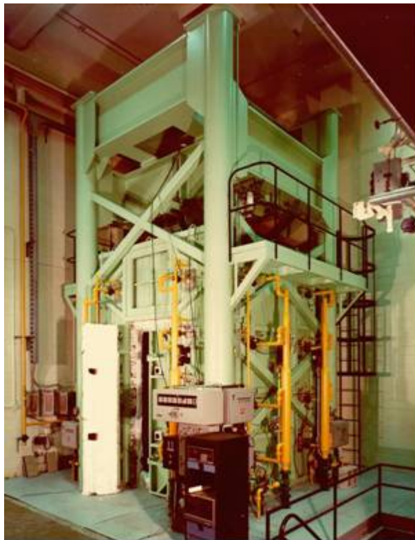
Figure 4. NRC full-scale column furnace for testing loaded columns.
