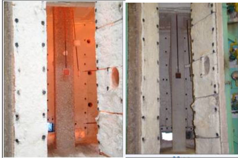
Figure 17. Column Specimens just after shutting down the burners of the furnace; E1259 test on the left and E119 test on the right.
