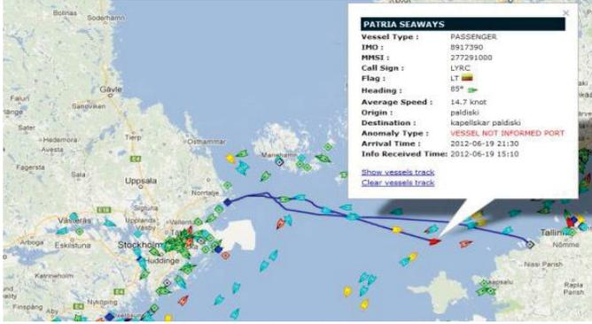
Fig. 1: Anomaly detection based on automatic identification system data (courtesy of Google)
