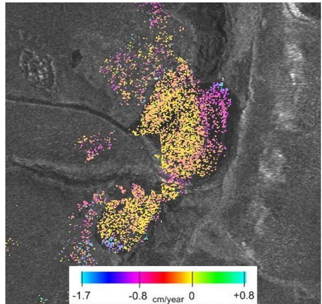
Fig. 5. Deformation map of the same two landfills shown in Figs 3 and 4 suggesting a subtle subsidence or sliding of the sides the landfill. RADARSAT-2 Data and Products ©MacDonald, Dettwiler and Associates Ltd. (2012) - All Rights Reserved. RADARSAT is an official mark of the Canadian Space Agency.
