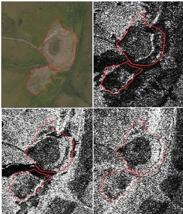
Fig. 3. Water ponding is visible at two landfills (outlined in red) at BAR-2 from the spring melt. CW from upper left are the Applanix airborne imagery from 3 Aug 2012, and radar backscatter from 24 May, 4 Aug and 17 June 2012 (all descending passes). RADARSAT-2 Data and Products ©MacDonald, Dettwiler and Associates Ltd. (2012) - All Rights Reserved. RADARSAT is an official mark of the Canadian Space Agency.
