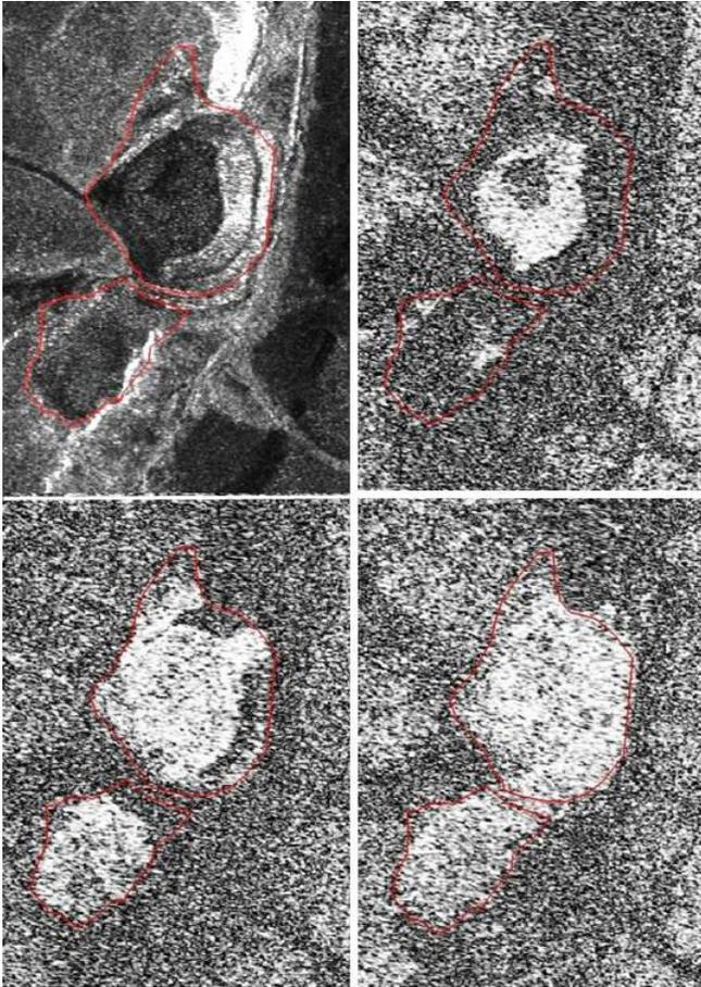
Fig. 4. Water ponding at two of the landfills (outlined in red) at BAR-2 from the Spring melt as observed (clockwise from upper left) in mean backscatter image, the coherence(27 May – 17 June), coherence(4 – 28 August) and the coherence(17 June – 11 July), all acquired in 2012. RADARSAT-2 Data and Products ©MacDonald, Dettwiler and Associates Ltd. (2012) - All Rights Reserved. RADARSAT is an official mark of the Canadian Space Agency.
