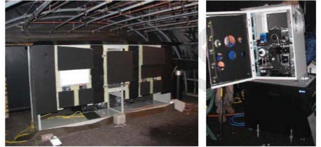
Fig. 6. Deployed target structure and camera box.
