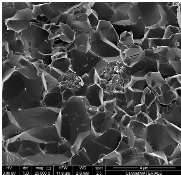
Figure 4b – Hot-pressed 1wt% SWCNT-O- $\text{Al}_2\text{O}_3$ (BM)
