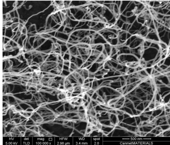
Figure 2b – Enlarge view of the MWCNTs
