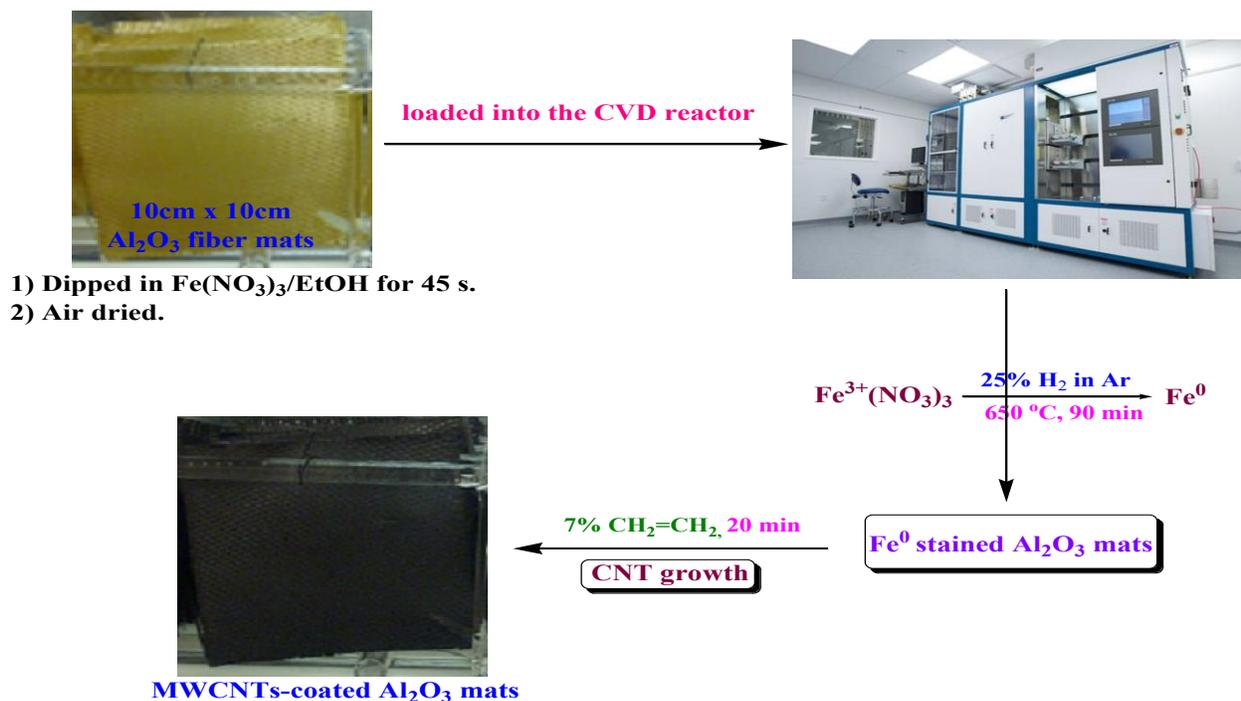
Figure 1 - Vertically grown MWCNTs on Al<sub>2</sub>O<sub>3</sub> fiber mat
