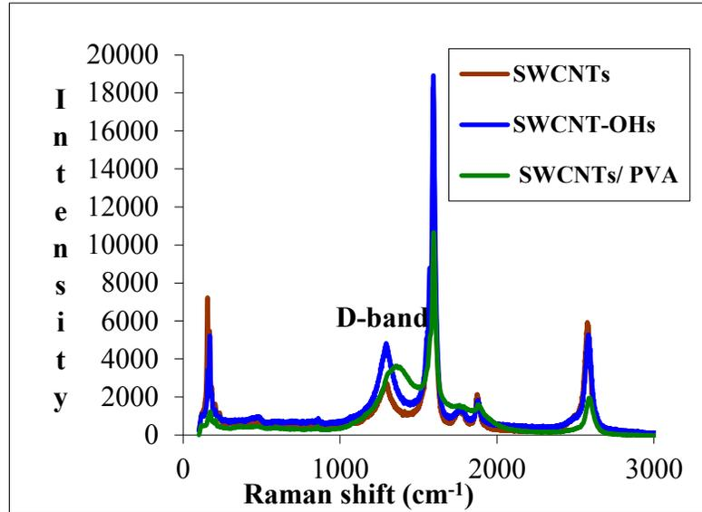
Figure 3b – Raman spectra of SWCNTs, SWCNT-OHs, and SWCNTs/PVA
