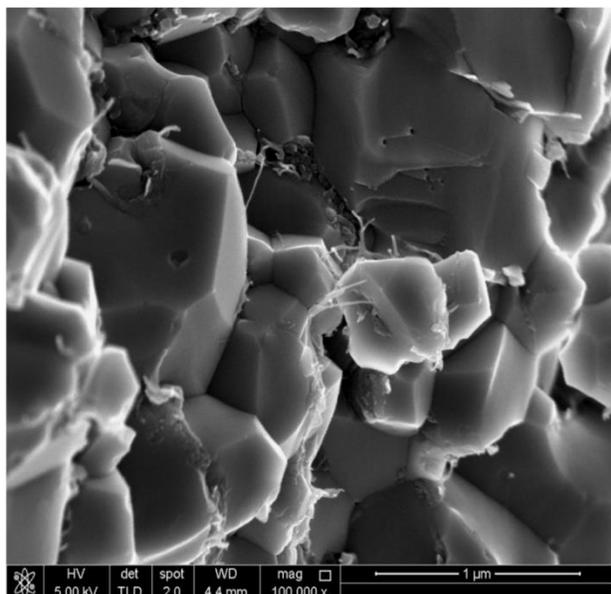
Figure 4a – Hot-pressed 1wt% SWCNT-O- $\text{Al}_2\text{O}_3$ (SP)
