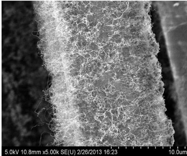
Figure 2a - MWCNTs grown on  $\text{Al}_2\text{O}_3$  fiber mat
