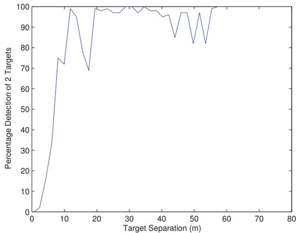
Figure 11. Probability of detection of 2 distinct targets. SNR=5dB.
