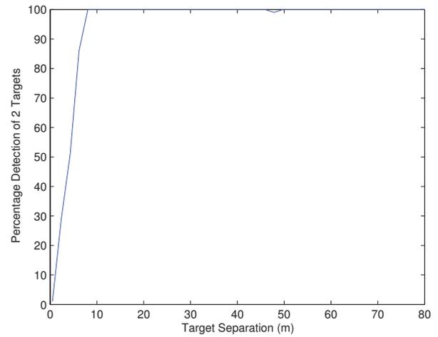
Figure 5. Probability of detection of 2 distinct targets. SNR=20dB.
