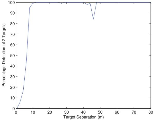
Figure 8. Probability of detection of 2 distinct targets. SNR=10dB.
