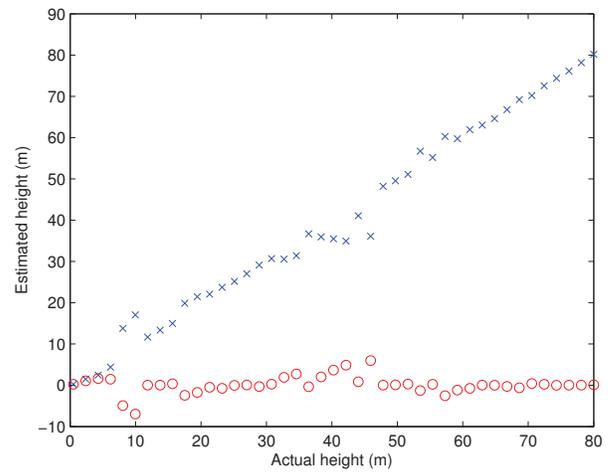
Figure 6. Estimated elevation positions, SNR=10 dB. Red o's denote estimated positions of the target at 0m elevation. Blue x's denote the estimated position of the second target.
