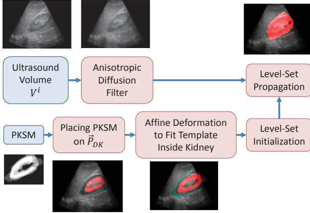
Fig. 3. Displaying the block diagram of our proposed kidney segmentation.
