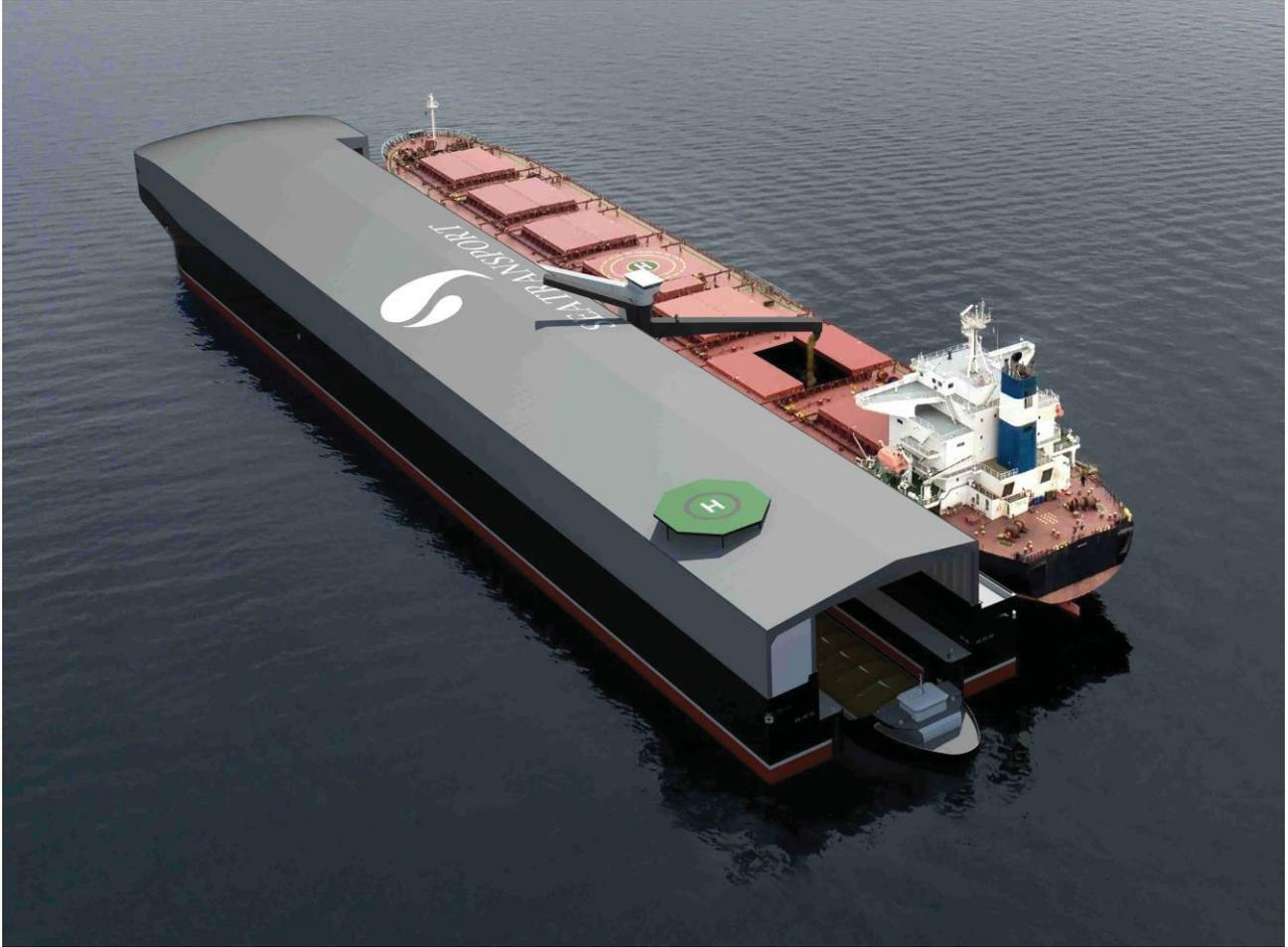
**Figure 1:** The floating harbour transhipper concept. The bow of the feeder vessel of up to 10,000 dwt capacity (foreground) protrudes from the stern well dock of the FHT (grey, centre). A Capesize export vessel is moored alongside (red and white, background). The FHT provides the offloading equipment to transfer the ore from the feeder vessel to the FHT, or from the FHT to the export vessel as shown here.
