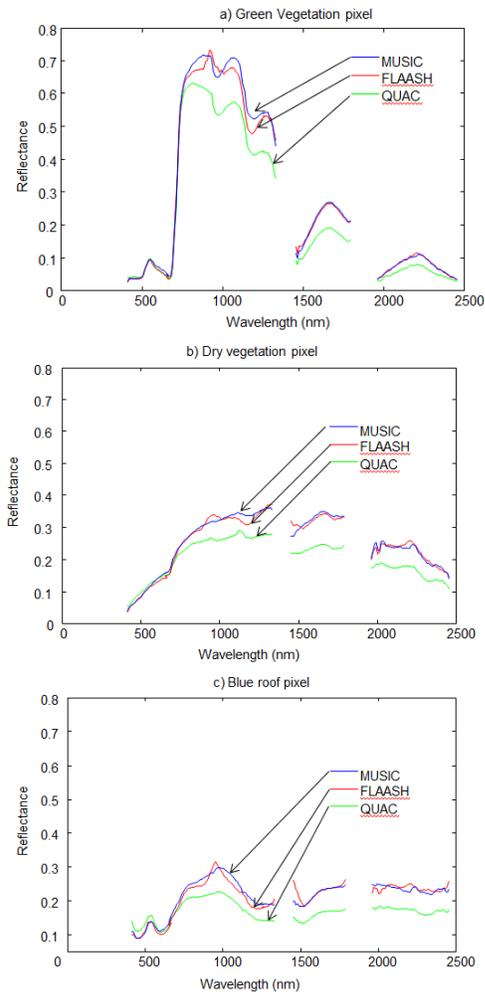
Figure 2: Comparison of reflectance spectra extracted by MUSIC, QUAC and FLAASH from an Aviris image
