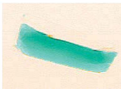
Figure 12. PC simulant Z_{eff} = 14.51 \pm 3.4\%
