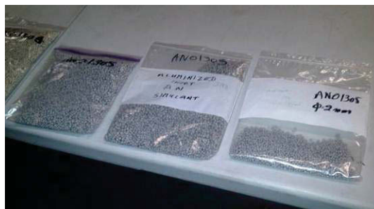
Figure 8. ANAL simulants with different prill sizes.
