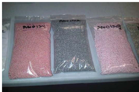
Figure 6. From the left, AN simulants 1301 and 1302, and ANAL simulant 1303.
