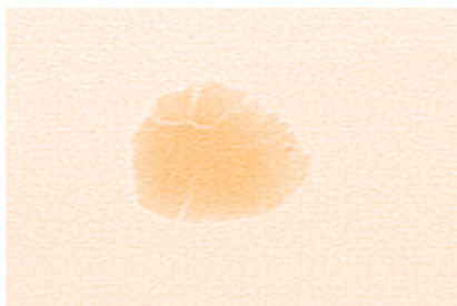
Figure 16. TATP in polyisobutylene matrix Z_{\text{eff}} = 6.46 \pm 2.8\%
