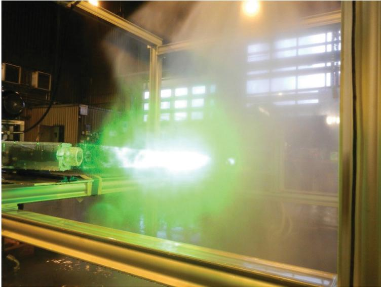
We measured the droplet size distribution as a function of system pressure. Pressure at the nozzle will be reduced in case of battle damage.
