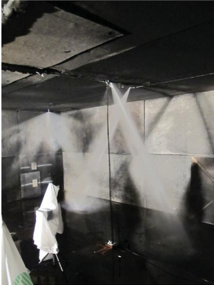
Spray of a regular watermist nozzle in the back and sprays from fragment holes in the front.
