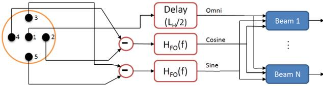
Fig. 6: Flow of data from hydrophones to beamformer 1 to N outputs.
