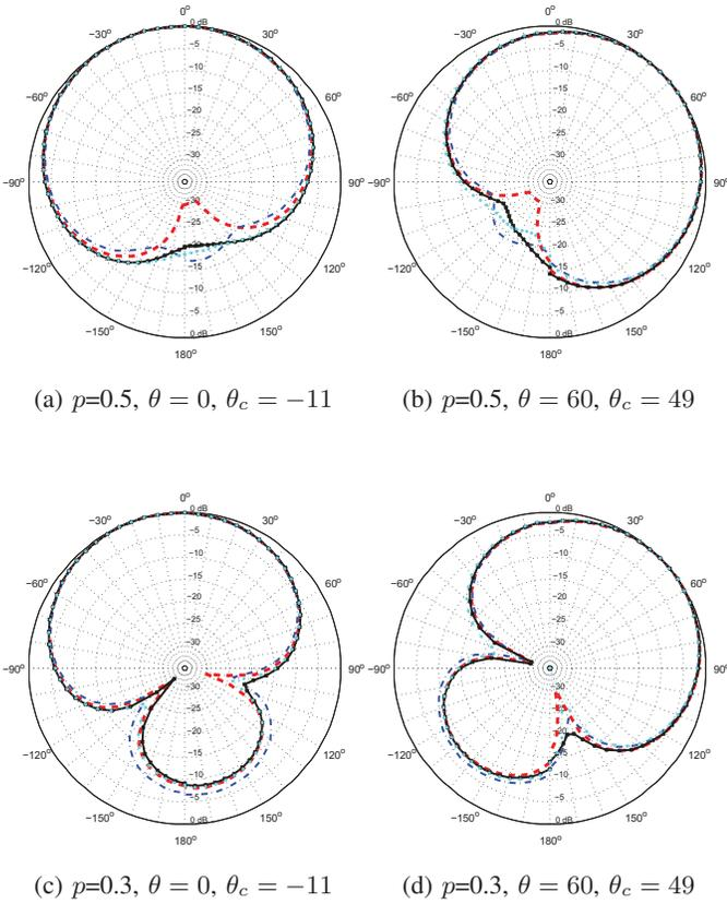
Fig. 9: Polar patterns measured using short, constant frequency pulses. Red is the ideal response, blue is the measured 2 kHz pattern, black is the measured 5 kHz pattern and turquoise is the measured 9 kHz pattern.
