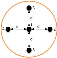
Fig. 4: 5-element array configuration. Each hydrophone is numbered and  $d$  is the spacing from the central hydrophone.
