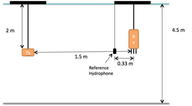
Fig. 7: Side view of the experimental deployment.
