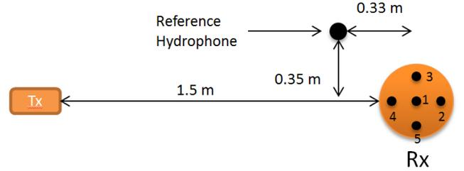
Fig. 8: Bottom view of the experimental deployment.
