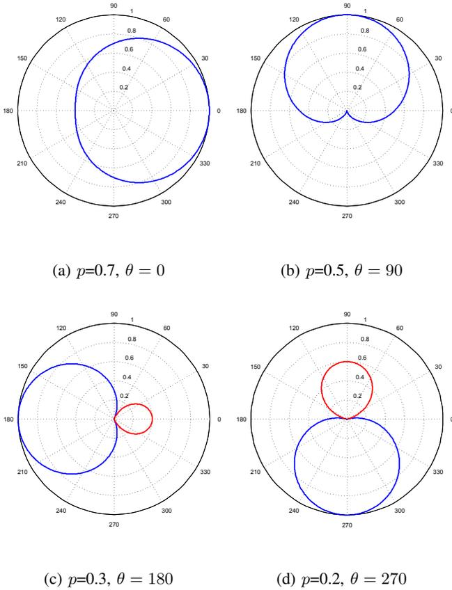
Fig. 3: Polar patterns of the beamformer for different pattern values,  $p$ , and azimuthal angles,  $\theta$ . Blue indicates in phase, red indicates out of phase or shifted by  $\pi$ .
