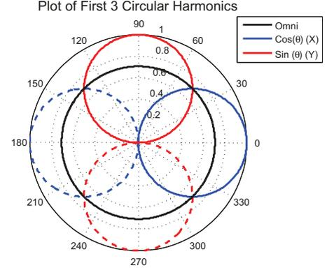
Fig. 2: Zeroth and first order circular harmonics. Dashed line indicates phase shift of  $\pi$ .
