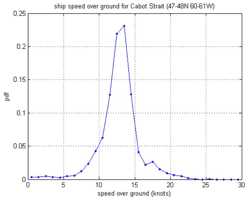
Figure 3. Probability density function of AIS transmitted speed over ground for ships near the west side of the Cabot Strait.
