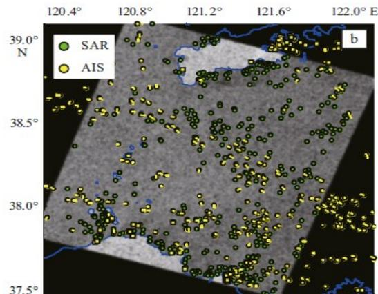
Figure 2. Example for RADARSAT-2 detected ship positions and AIS ship positions (adopted from Ji et al., 2014).
