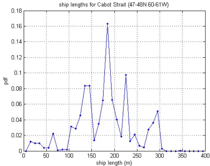
Figure 5. Probability density function of AIS transmitted ship lengths for ships near the west side of the Cabot Strait.
