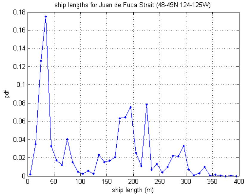
Figure 8. Probability density function of AIS transmitted ship lengths for ships near the entrance to the Juan de Fuca Strait.
