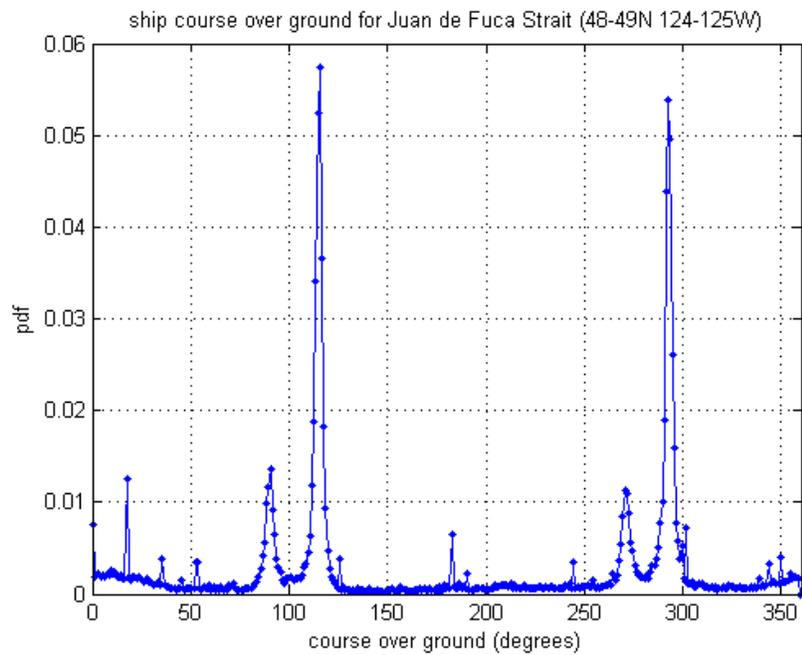
Figure 7. Probability density function of AIS transmitted course over ground for ships near the entrance to the Juan de Fuca Strait.
