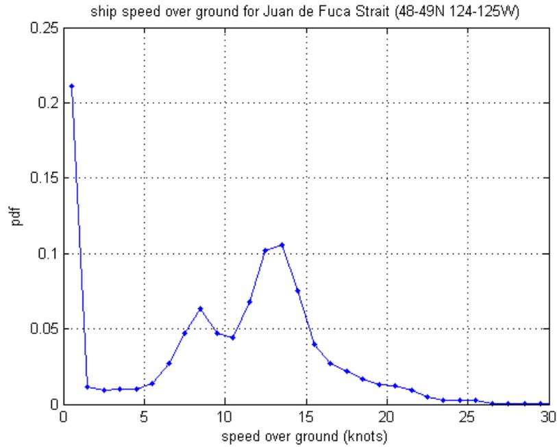
Figure 6. Probability density function of AIS transmitted speed over ground for ships near the entrance to the Juan de Fuca Strait.
