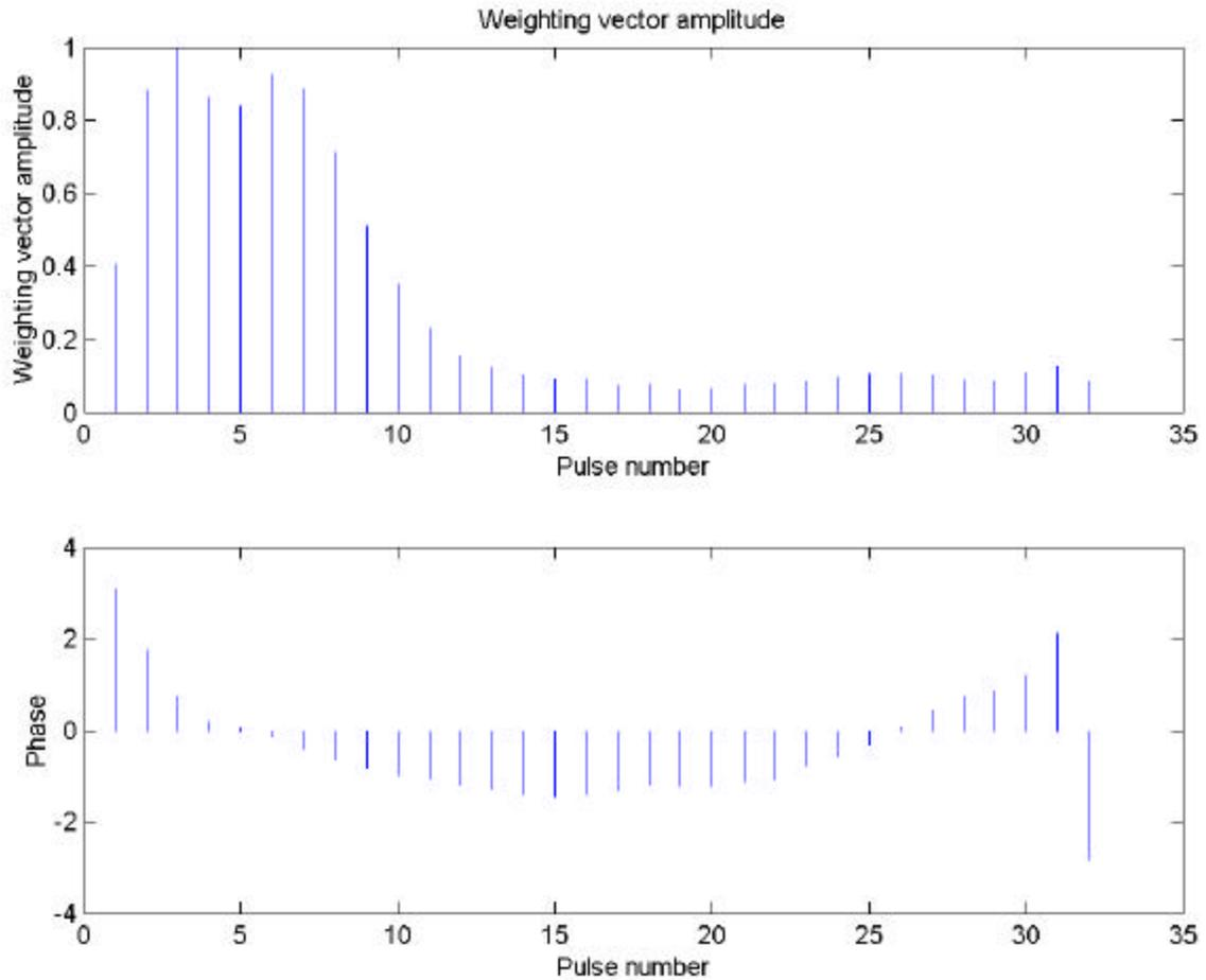
**Figure 4 Optimal weighting vector at the end of 30 iterations of amplitude-constrained waveform design with constant amplitude zero phase initial burst**
