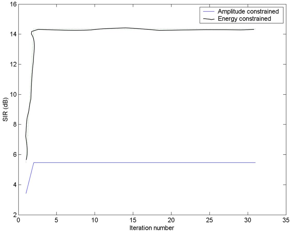
**Figure 19 SIR values obtained by amplitude-constrained and energy-constrained waveform design at only iteration 1 with constant amplitude zero phase initial burst**
