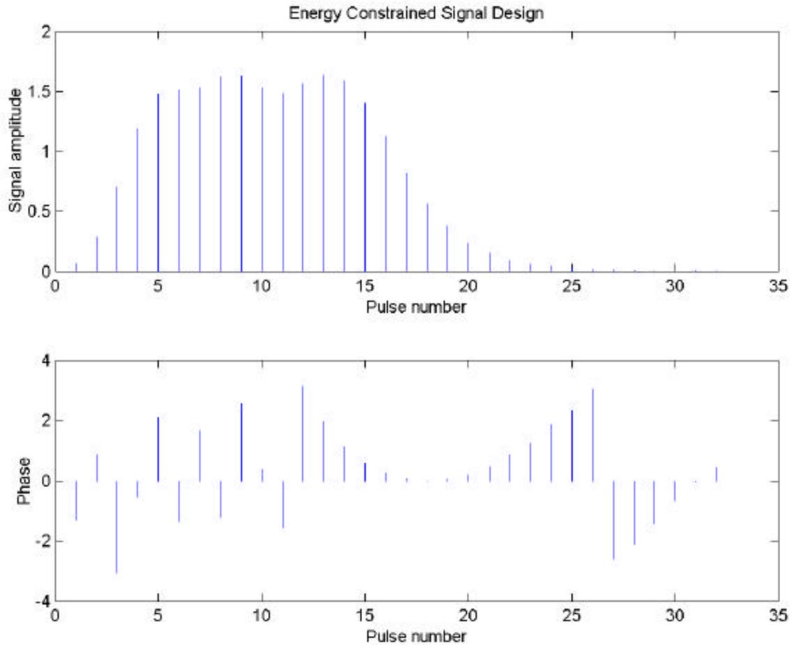
**Figure 9** Pulse train at the end of 30 iterations of energy-constrained waveform design with constant amplitude quadratic phase initial burst
