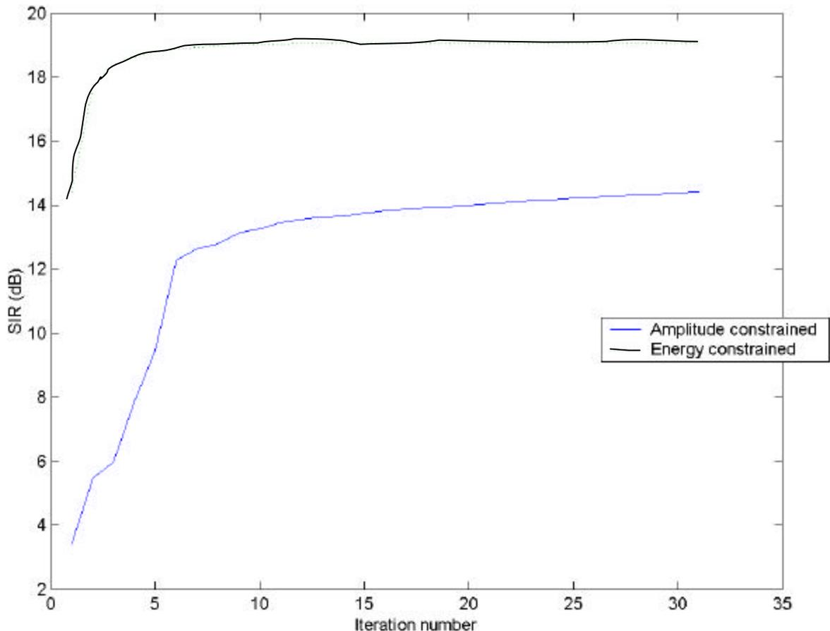
**Figure 2 SIR values obtained by amplitude-constrained and energy-constrained waveform design with constant amplitude zero phase initial burst**
