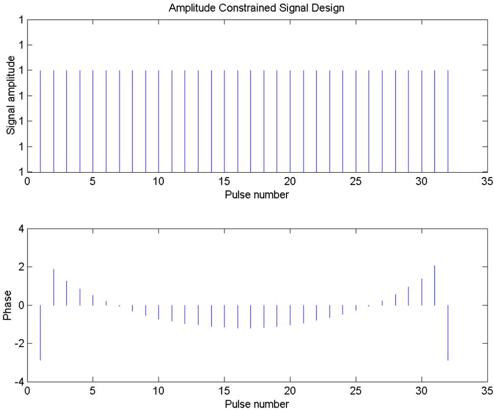
**Figure 14** Pulse train at the end of 30 iterations of amplitude -constrained waveform design with constant amplitude zero phase initial burst (single-pulse SNR = -15dB)
