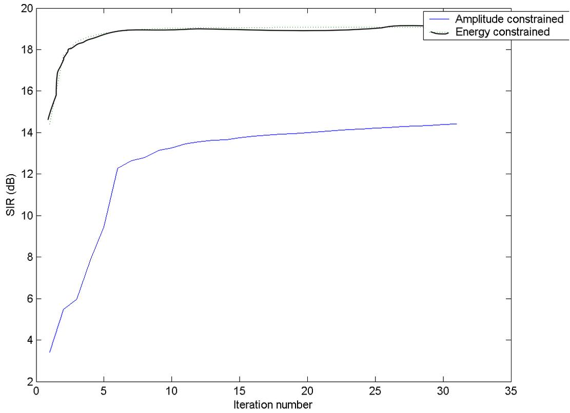
**Figure 16 The SINR values obtained with the modified target-clutter environment**
