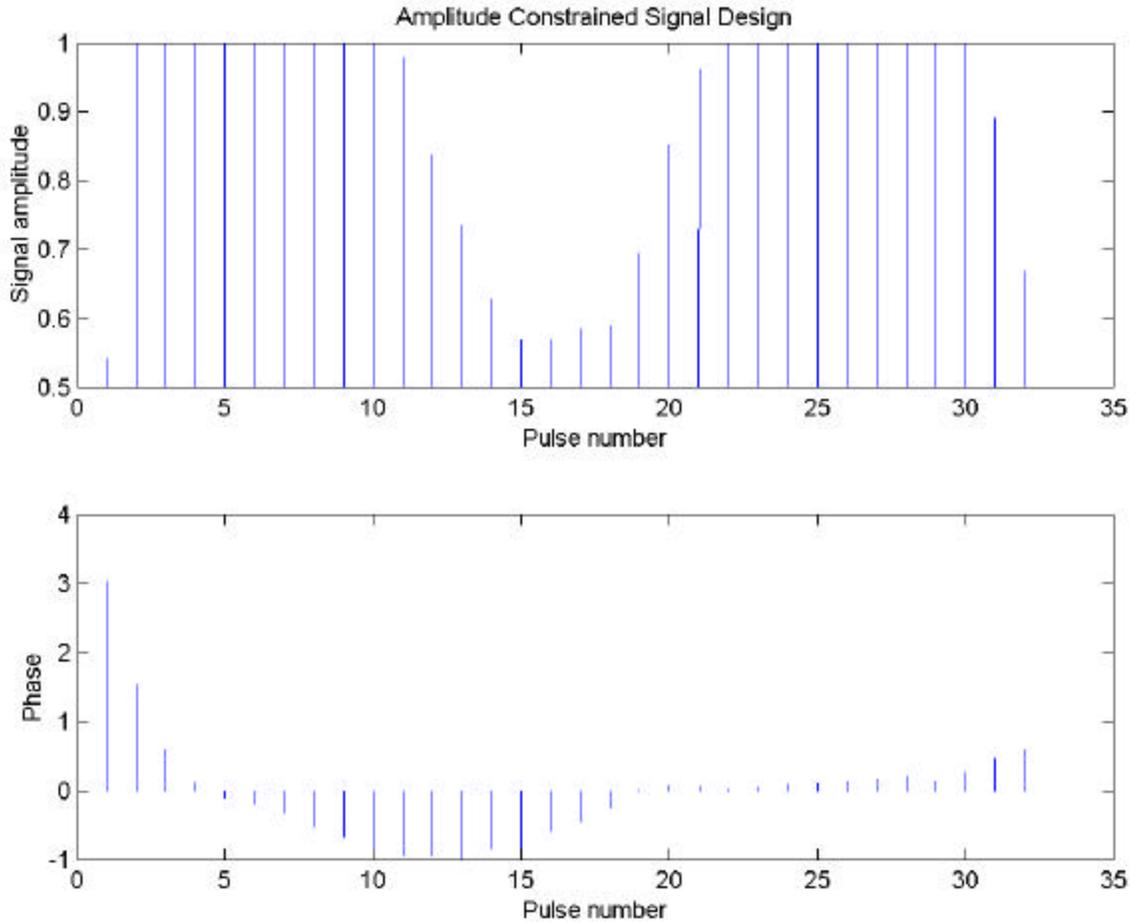
**Figure 3 Pulse train at the end of 30 iterations of amplitude-constrained waveform design with constant amplitude zero phase initial burst**
