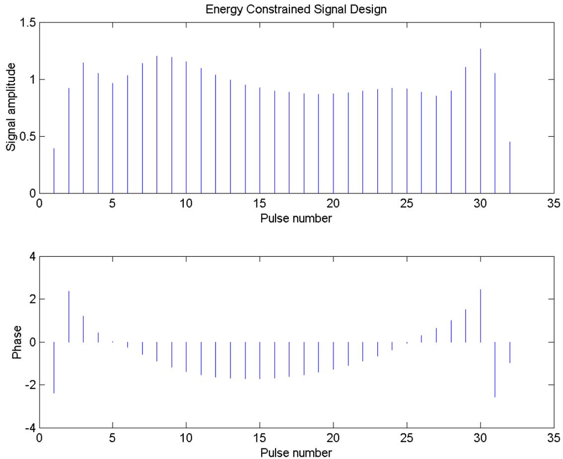
**Figure 12 Pulse train at the end of 30 iterations of energy-constrained waveform design with constant amplitude zero phase initial burst (single-pulse SNR = -5dB)**
