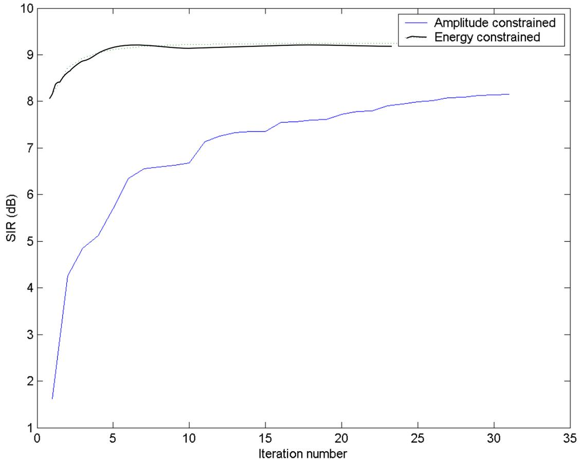
**Figure 10 SIR values obtained by amplitude-constrained and energy-constrained waveform design with constant amplitude zero phase initial burst and single-pulse SNR of -5dB.**
