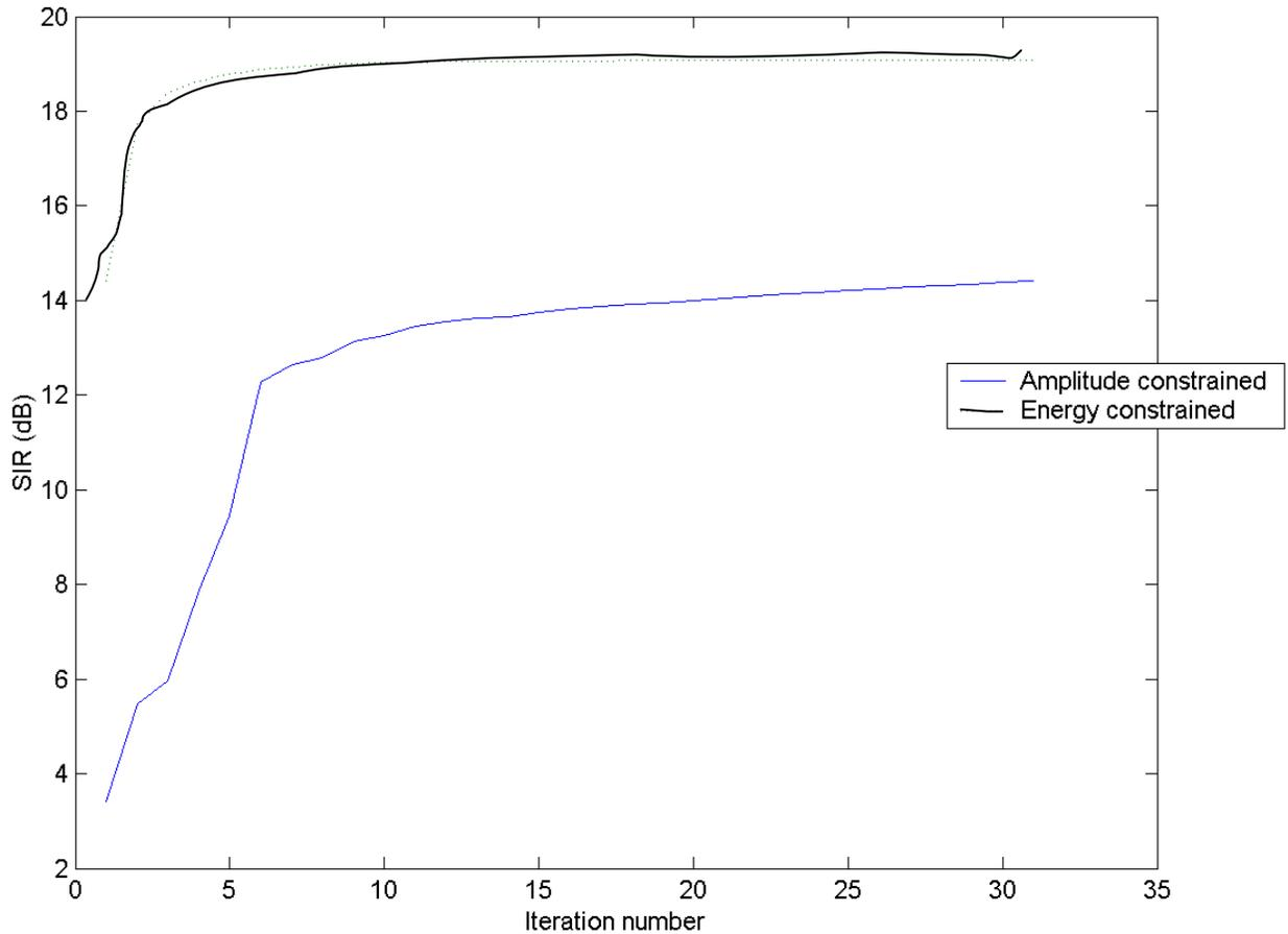
**Figure 18** The SINR values obtained with the modified target-clutter environment in **Figure 17**
