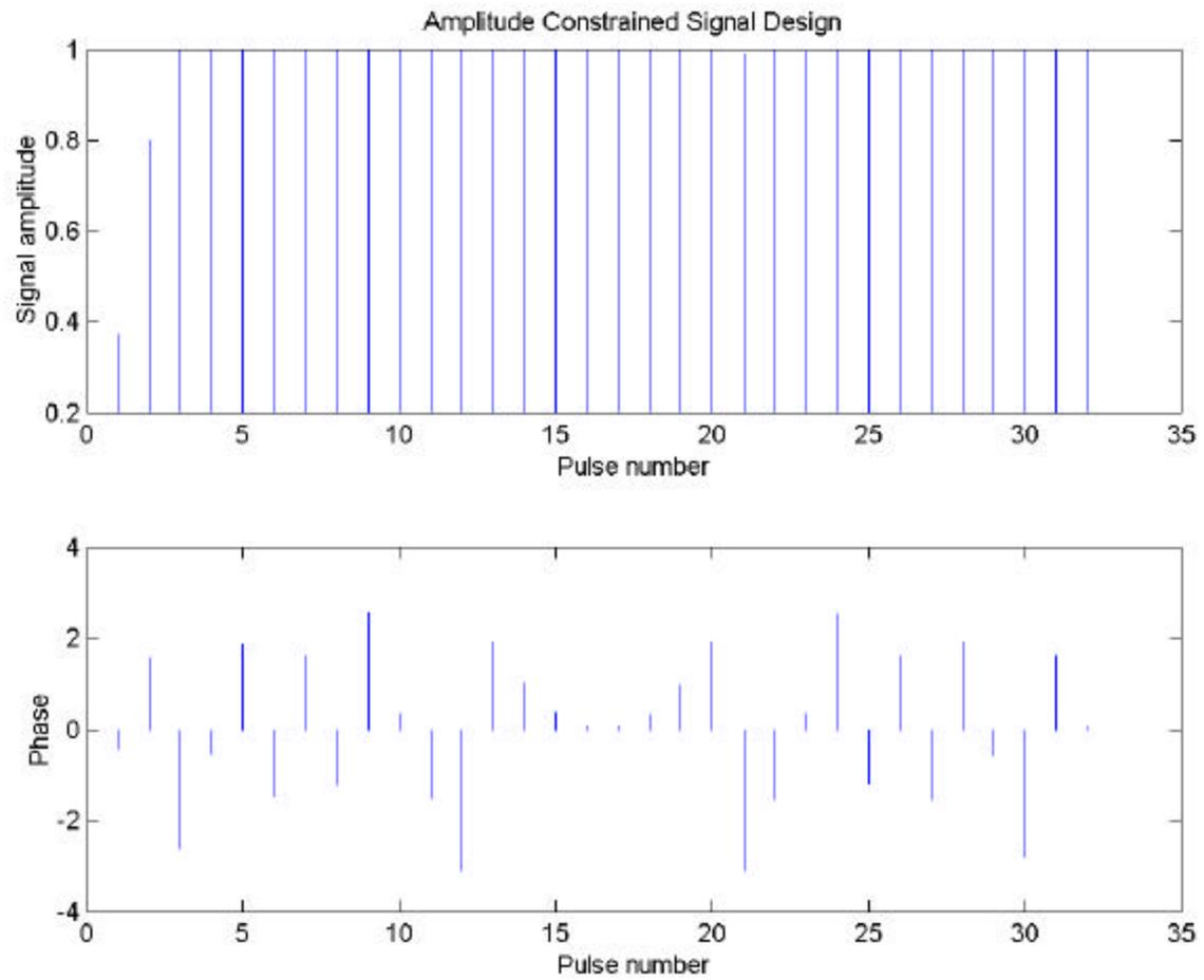
**Figure 7 Pulse train at the end of 30 iterations of amplitude-constrained waveform design with constant amplitude quadratic phase initial burst**
