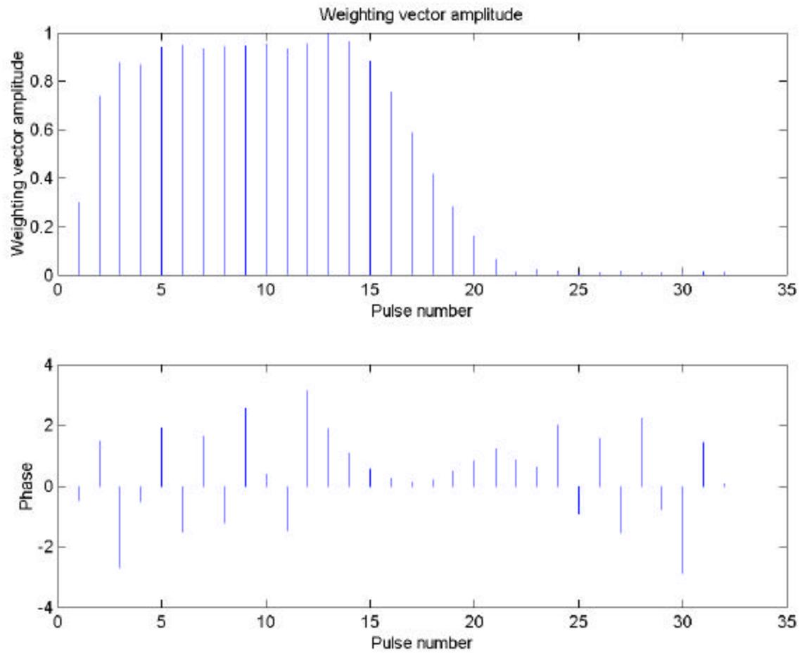
**Figure 8 Optimal weighting vector at the end of 30 iterations of amplitude-constrained waveform design with constant amplitude quadratic phase initial burst**
