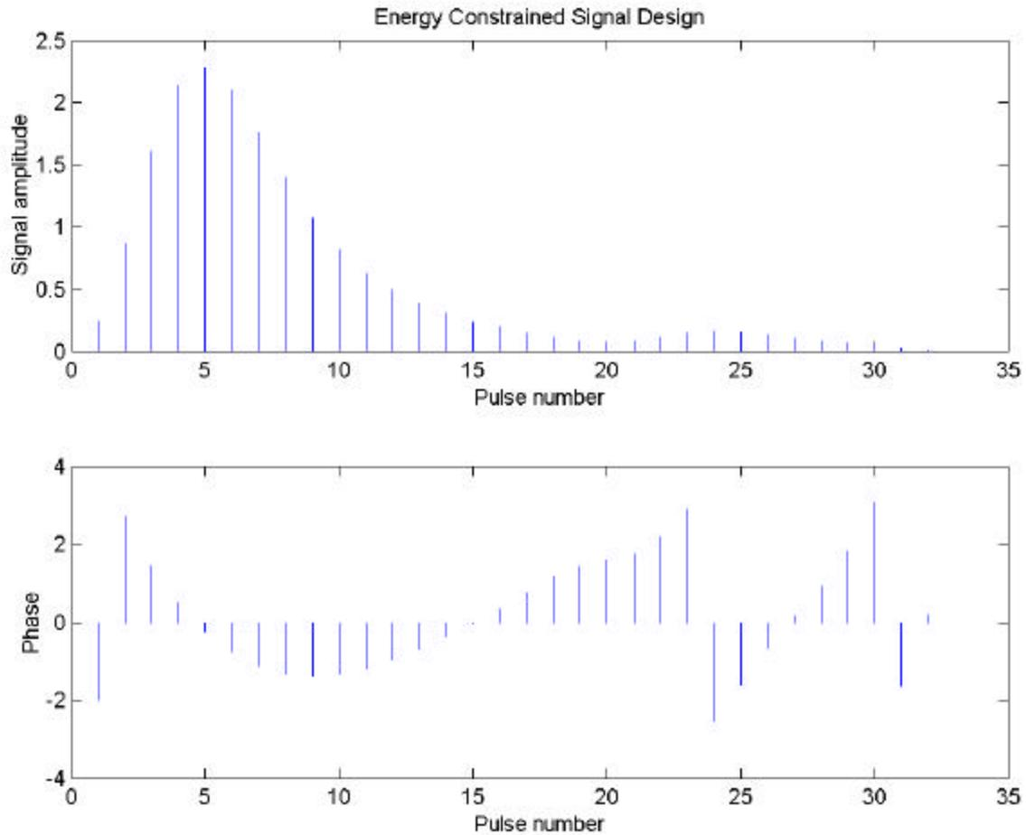
**Figure 5 Pulse train at the end of 30 iterations of energy-constrained waveform design with constant amplitude zero phase initial burst**
