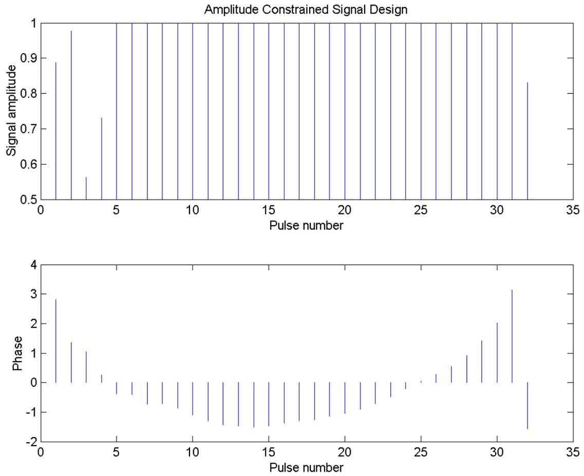
**Figure 11 Pulse train at the end of 30 iterations of amplitude -constrained waveform design with constant amplitude zero phase initial burst (single-pulse SNR = -5dB)**
