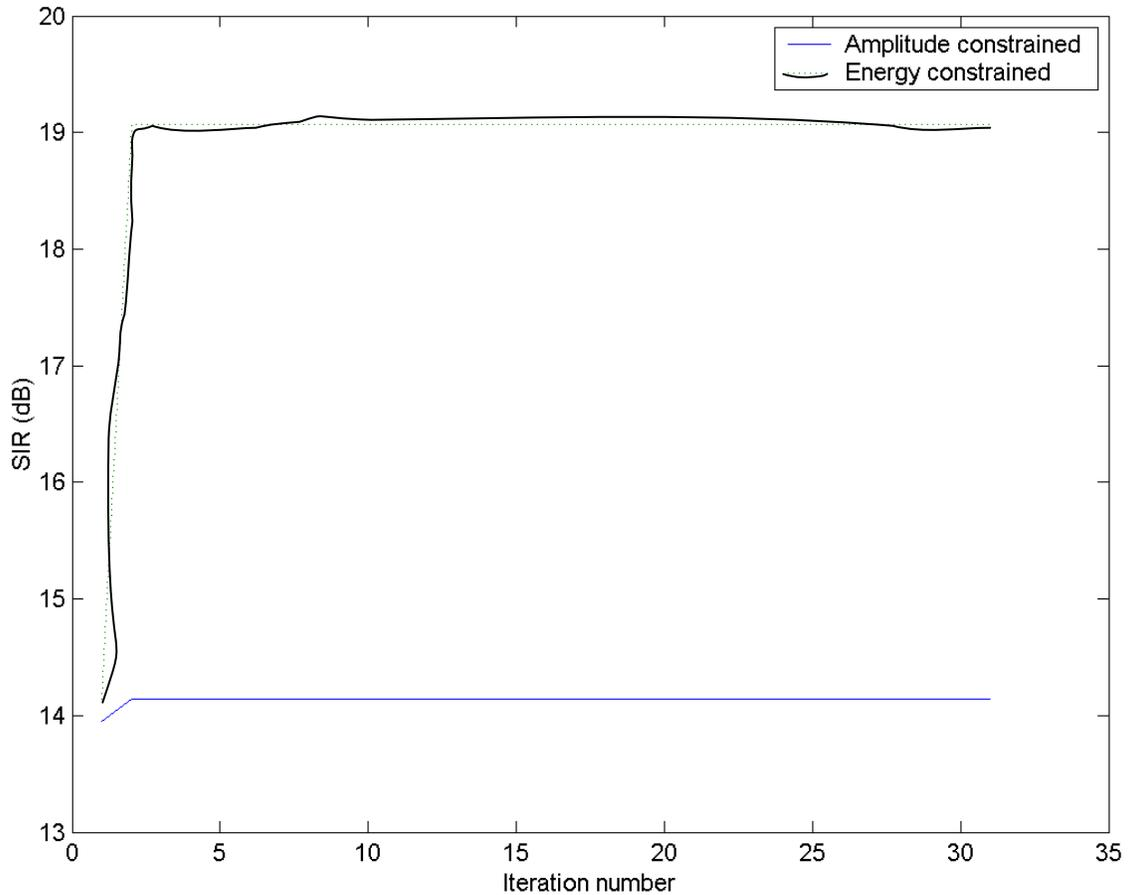
**Figure 20 SIR values obtained by amplitude-constrained and energy-constrained waveform design at only iteration 1 with constant amplitude quadratic phase initial burst**
