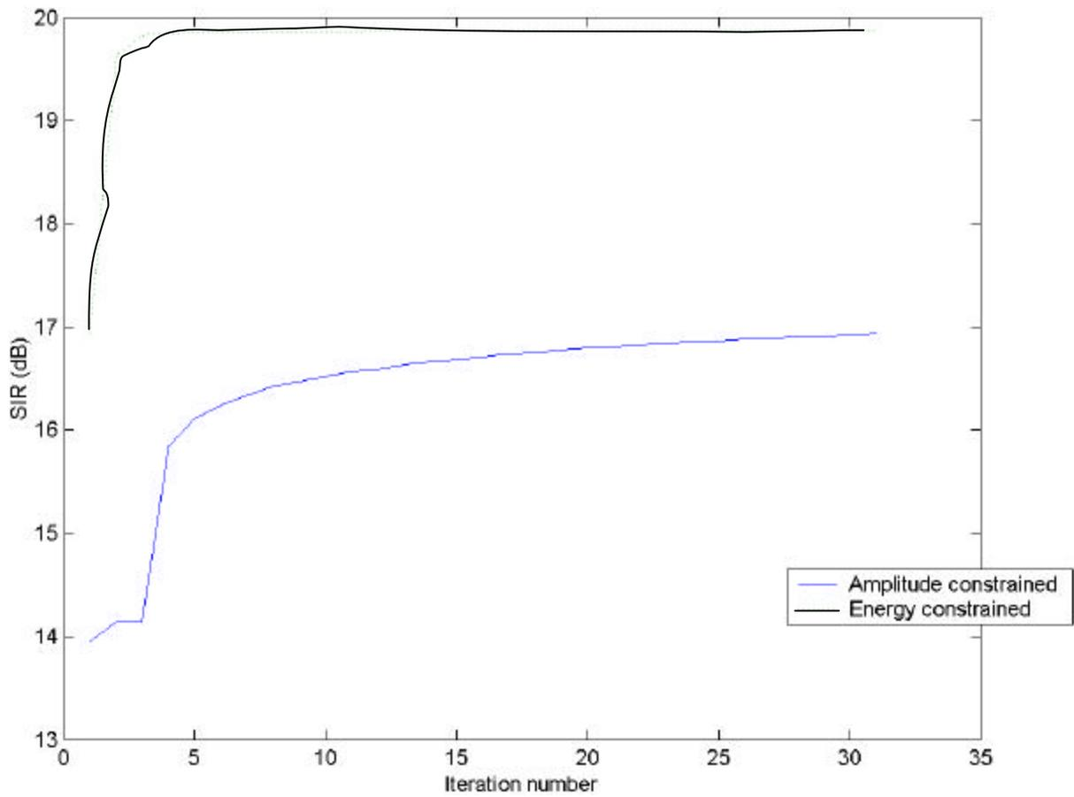
**Figure 6** SIR values obtained by amplitude-constrained and energy-constrained waveform design with constant amplitude quadratic phase initial burst
