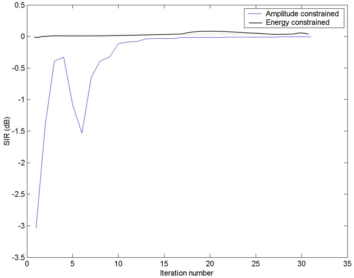
**Figure 13 SIR values obtained by amplitude-constrained and energy-constrained waveform design with constant amplitude zero phase initial burst and single-pulse SNR of -15dB.**
