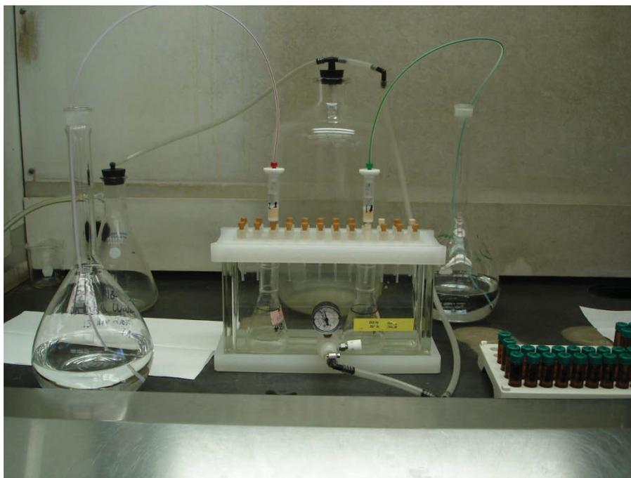
*Figure 1: Extraction setup*
