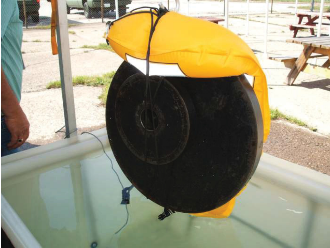
Figure 2 CF Jet Aircrew LP/SV Bladder Attached to One 45lb and One 10 lb Plate That Are Acting to Counter The Buoyant Force. (35g CO 2 canister test)
