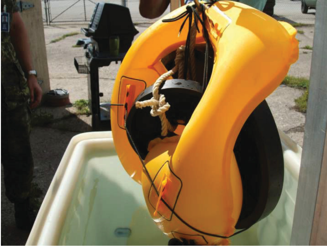
Figure 5 CF Jet Aircrew LP/SV Bladder using a 45g CO 2 canister.
