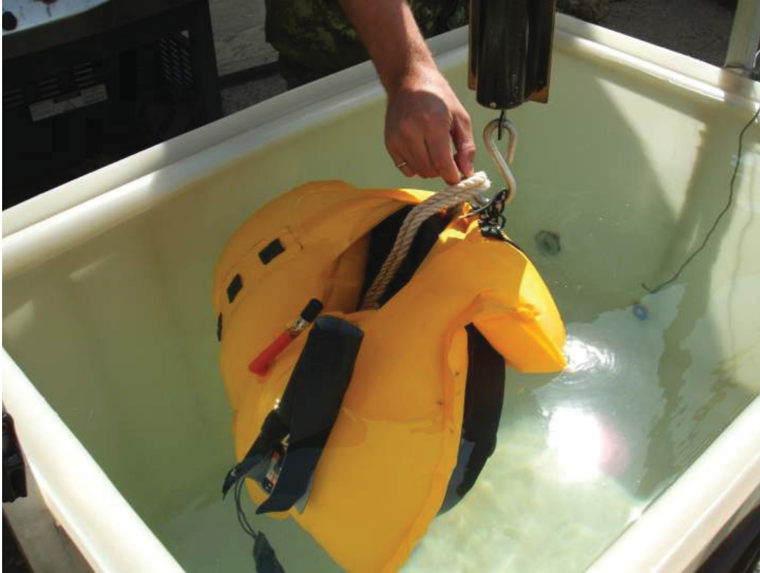
Figure 4 British MK 30 LCX Bladder Buoyancy Test using 35g CO 2 canister. Note that the hand in the photo was not producing any force in the vertical direction, it was simply ensuring that the connecting rope remained hooked on the spring scale.
