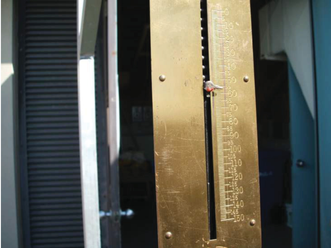
Figure 3 Chatillon Type 100 Spring Scale Measurement Intervals
