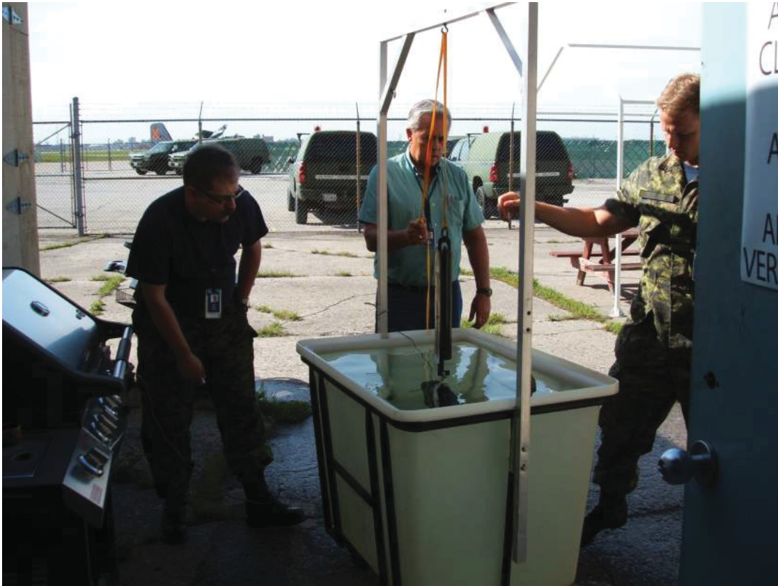
Figure 1 Determining Submersed Weight of 45lb Plate
