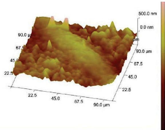
Fig. 7. A 3-dimensional surface view on white-etching band region in maraging steel 300
