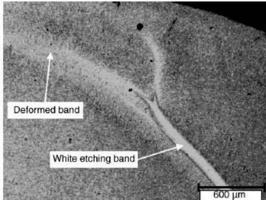
Fig. 1. Optical micrograph showing a white etching (transformed) band and a deformed band in the microstructure of a steel specimen after impact [2].
