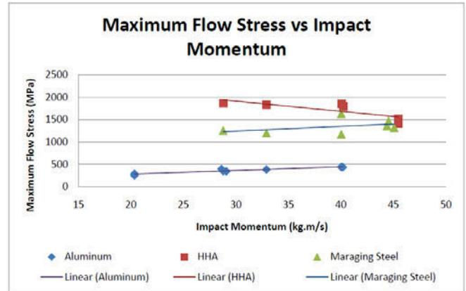
Fig. 4. The effect of impact momentum on maximum flow stress for all three metals
