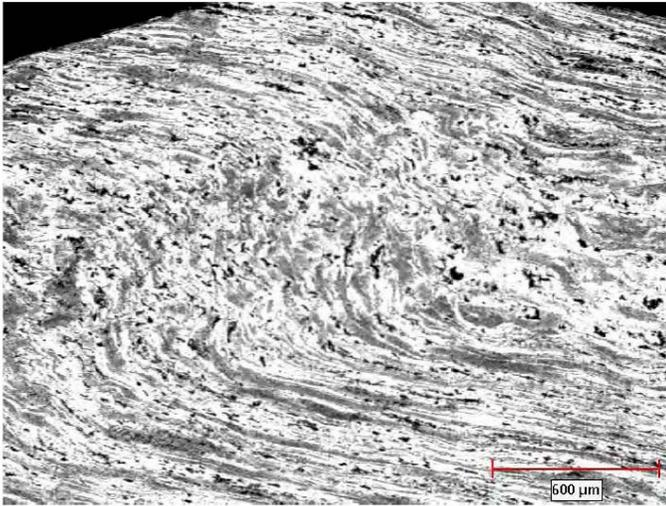
Fig. 6. Aluminum specimen impacted at 28.63 kg.m/s showing deformed band
