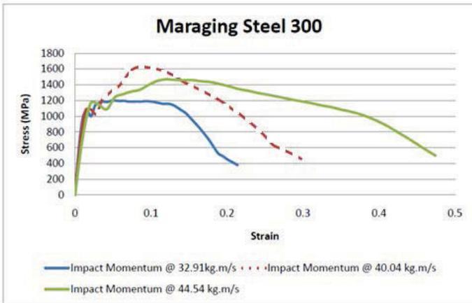
Fig. 3. Typical dynamic stress-strain responses for maraging steel 300 specimens at different impact momenta
