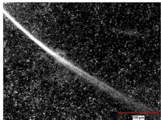
Fig. 5. Maraging steel 300 specimen impacted at 44.54 kg.m/s showing deformed and white etching bands
