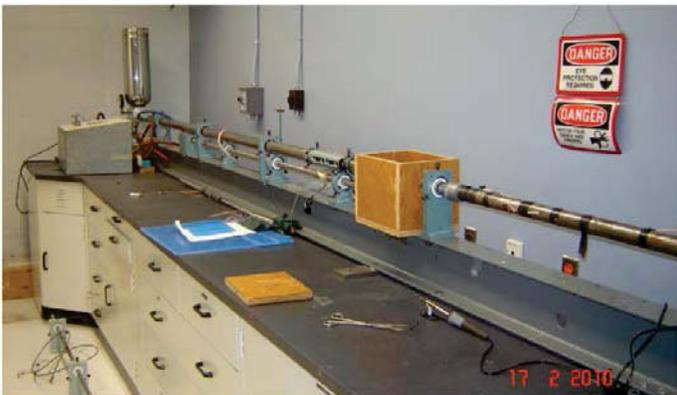
Fig. 2. Direct Impact Split Hopkinson Pressure Bar at The University of Manitoba
