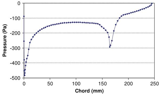
**Figure 6.** Differential pressure profile for dash with AOA =  $0^\circ$ , Flap =  $20^\circ$ .
