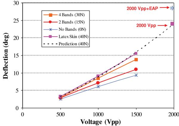
**Figure 10.** Effect of axial compressive load on MFC28.
