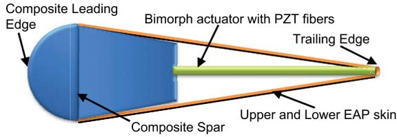
**Figure 2.** Cross-section of the dual actuator based smart wing design.
