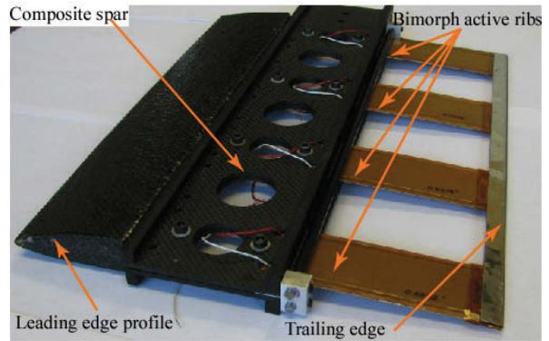
**Figure 8.** Smart wing hardware model.
