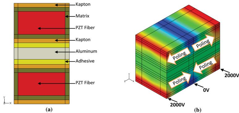
**Figure 7.** Finite element model (a) geometry and material with (b) voltage and polarization.
