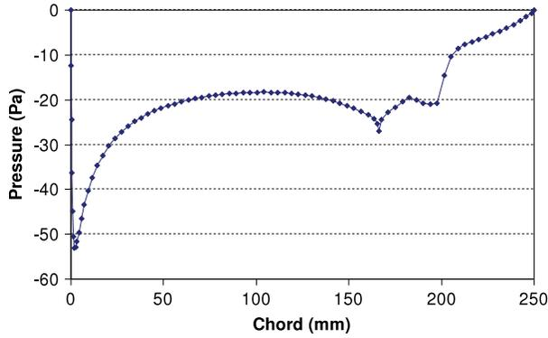
**Figure 5.** Differential pressure profile for dash with AOA =  $0^\circ$ , Flap =  $2^\circ$ .
