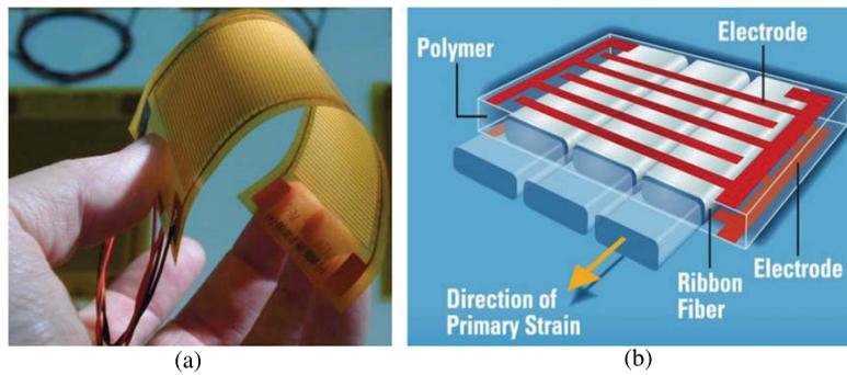
**Figure 3.** (a) Conformable piezoceramic fiber actuators and (b) schematic of the actuator design.
