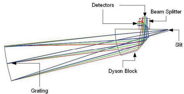
Figure 1. Layout of the optical design of the selected Dyson spectrometer
