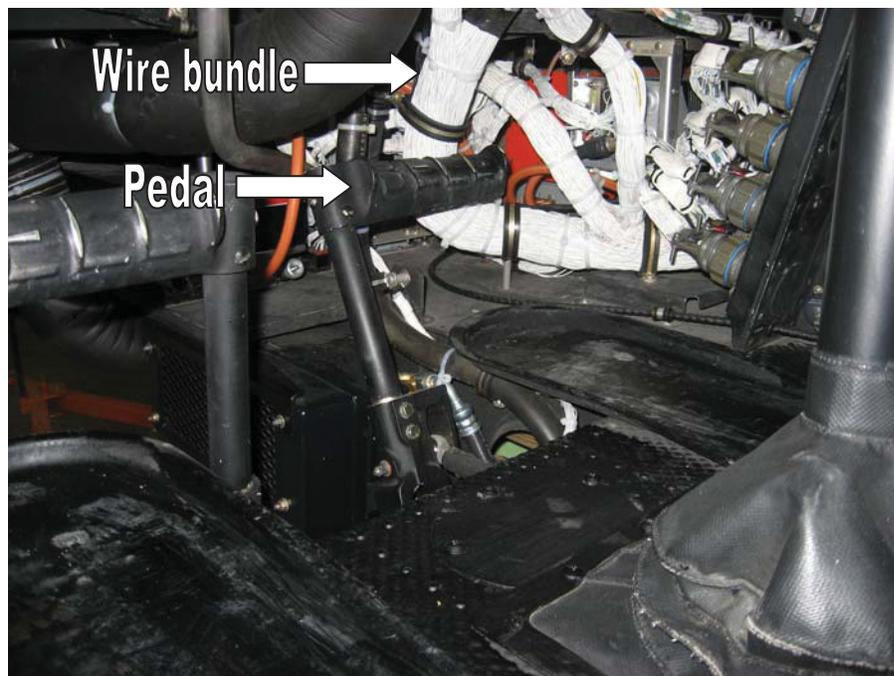
*Figure 1 Left seat pedals versus wire bundles routing*
