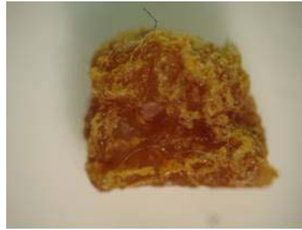
Figure 5: Microscopic photographs of a piece of GIM before (left) and after 47 weeks (right) in dripping test
