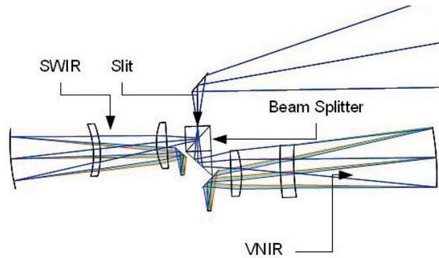
Figure 4. Layout of the optical design of imaging spectrometer option D.
