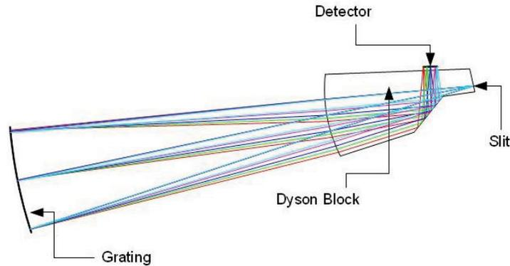
Figure 1. Layout of the optical design of imaging spectrometer option A.
