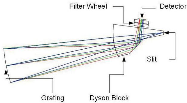
Figure 3. Layout of the optical design of imaging spectrometer option C.
