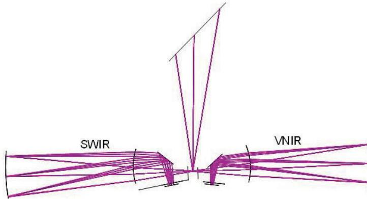
Figure 5. Layout of the optical design of imaging spectrometer option E.
