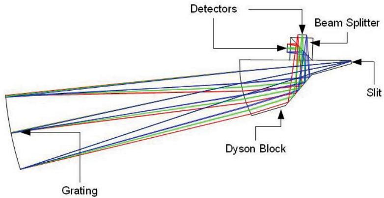
Figure 2. Layout of the optical design of imaging spectrometer option B.
