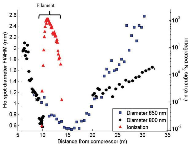
Fig. 4. (Color online) Hot spot diameters FWHM plotted as a function of the distance from the compressor. The black circles show the data measured using BP800 and the blue squares, the data obtained with BP850. The red triangles correspond to the fluorescence signal intensity measured along the beam with a PMT. The corresponding scale is on the right-hand side of the figure.
