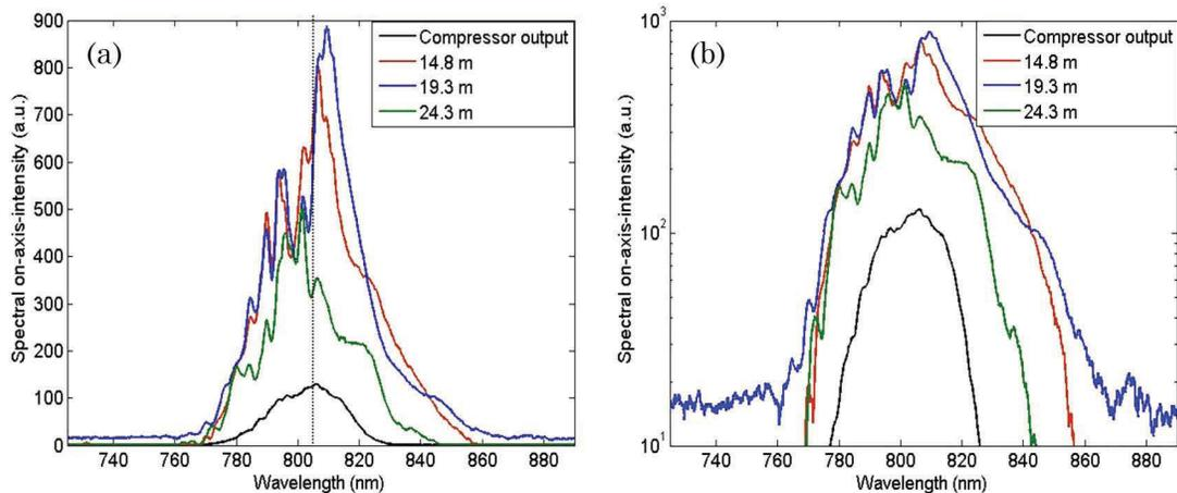
Fig. 2. (Color online) On-axis spectra measured using a fiber spectrometer coupled to an integration sphere. A 2.5 mm diameter pinhole ensured that only the filament/postfilament hot spot entered the sphere. Spectra are presented for different positions in (a) linear and (b) logarithmic scales.
