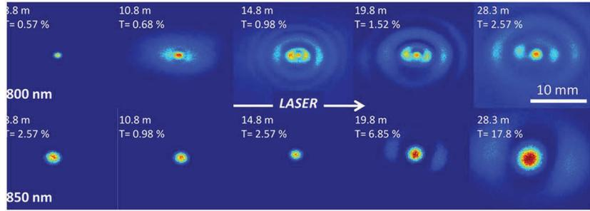
Fig. 3. (Color online) Beam patterns measured along the propagation direction using a CCD camera protected with bandpass filters centered at 800 nm (top row) and 850 nm (bottom row).
