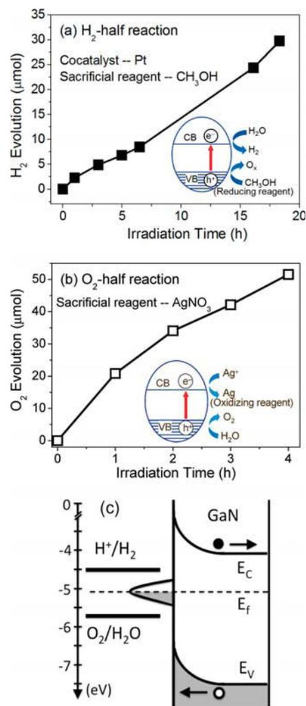
**Figure 2.** (a) H<sub>2</sub> and (b) O<sub>2</sub> evolution half-reactions in the presence of respective sacrificial reagents over GaN nanowires under a 300 W full arc xenon lamp irradiation. The corresponding reaction processes are schematically illustrated in the insets. (c) GaN surface defects pin the Fermi level at the surface and bend the bands upward, thereby driving holes to the nanowire sidewall and electrons into the bulk.
