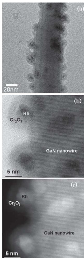
**Figure 3.** (a) Low magnification TEM image shows uniform distribution of the Rh/Cr<sub>2</sub>O<sub>3</sub> nanoparticles on GaN nanowire surfaces. (b) HRTEM image and (c) HR-HAADF image clearly show the Rh/Cr<sub>2</sub>O<sub>3</sub> core-shell nanostructures deposited on GaN nanowires.
