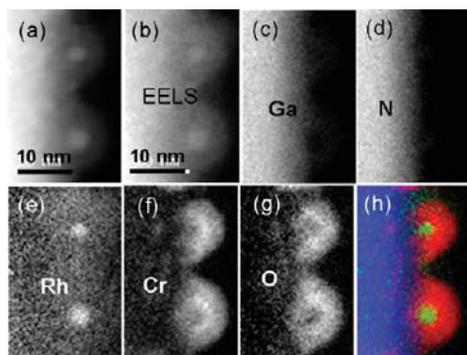
**Figure 4.** (a) HR-HAADF image and (b) EELS mapping image, (c–g) corresponding individual element mapping images, and (h) RGB image (red, Cr; green, Rh; blue, Ga), clearly showing the Rh/Cr<sub>2</sub>O<sub>3</sub> core-shell nanostructure deposited on GaN nanowires.
