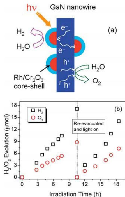
**Figure 5.** (a) Schematic illustration of water splitting on GaN nanowires with the incorporation of Rh/Cr<sub>2</sub>O<sub>3</sub> core-shell nanostructures as cocatalysts. (b) Experimental overall photocatalytic water splitting on Rh/Cr<sub>2</sub>O<sub>3</sub> core-shell nanostructure deposited GaN nanowires, under a 300 W full arc xenon lamp irradiation for a duration of 18 h. No degradation of the photocatalytic activity was observed during the course of two cycles of reaction.
