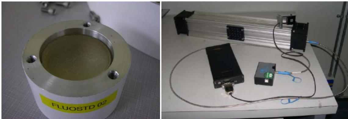
Figure 4 Picture of a calibration LIF target (left) and the optical setup (right) used to derive precisely the quantum yield of a calibration target as well as its spectral probability distribution.
