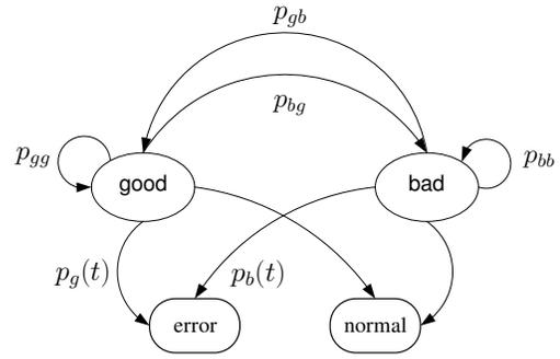
Fig. 1. State transition diagram of the proposed two-state Markov process.
