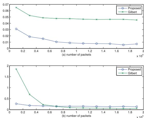
Fig. 6. RMSE of the estimated transition probabilities versus number of packets.
