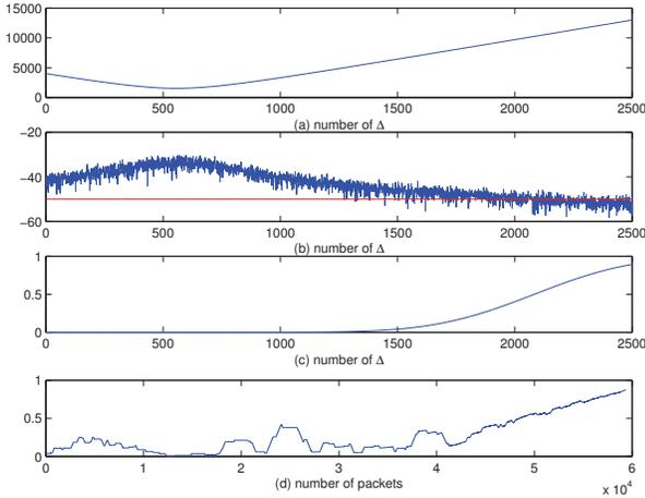
Fig. 2. Variation of error statistics of packet dropout versus distance between two UAVs.
