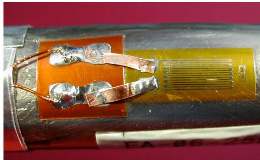
**Fig. 4.** Copper foil soldered to connection tab and the strain gage's tab with very thin wires
