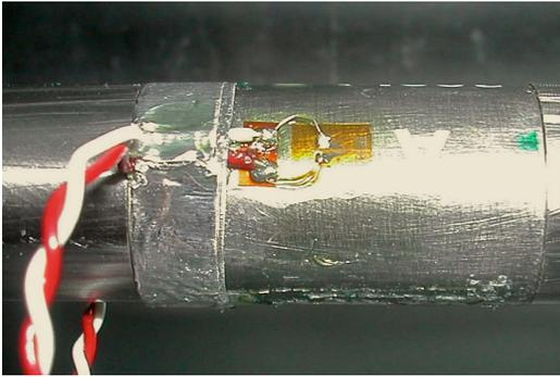
**Fig. 1.** Standard installation of strain gage before investigation
