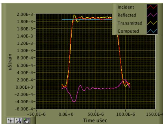
Fig. 7. HSR test result of Stress-Proof. Impact velocity of 21.9m/s.
