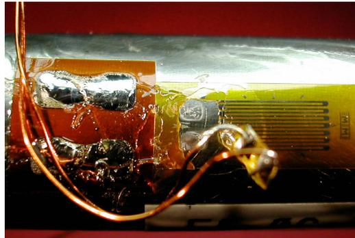
**Fig. 3.** Thin wires soldered to the strain gage's tab after failure
