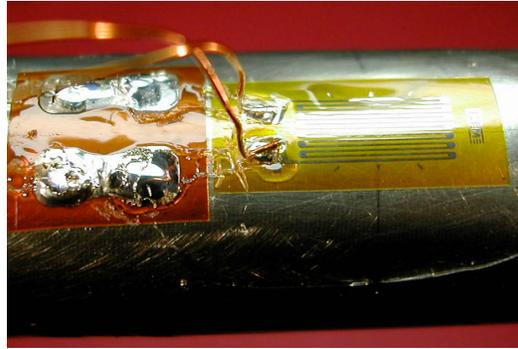
**Fig. 2.** Thin wires soldered to the strain gage's tab
