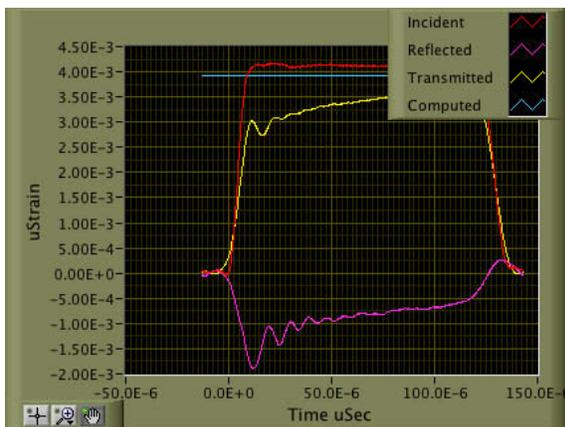
Fig. 8. HSR test result of Stress-Proof. Impact velocity of 37.3m/s
