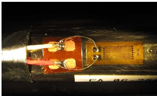
Fig. 6. Connection Tab soldering technique
