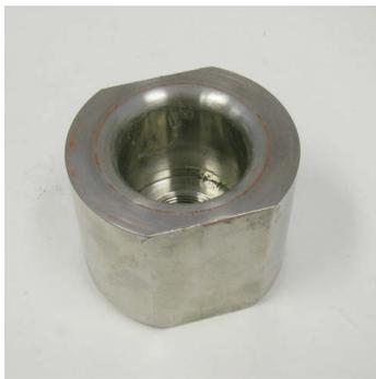
**Figure 6a.** Bottom portion of the mould.
