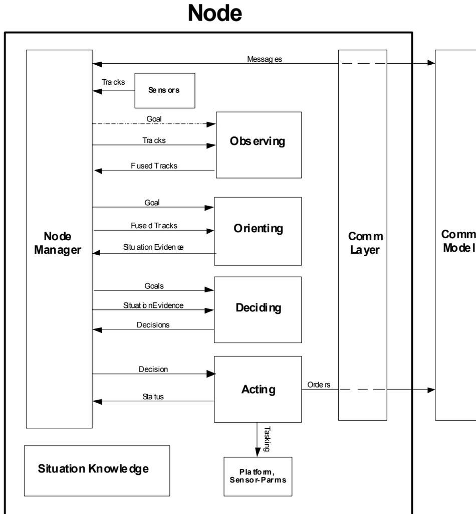
Figure 4 Internal OODA Structure of a Node.
