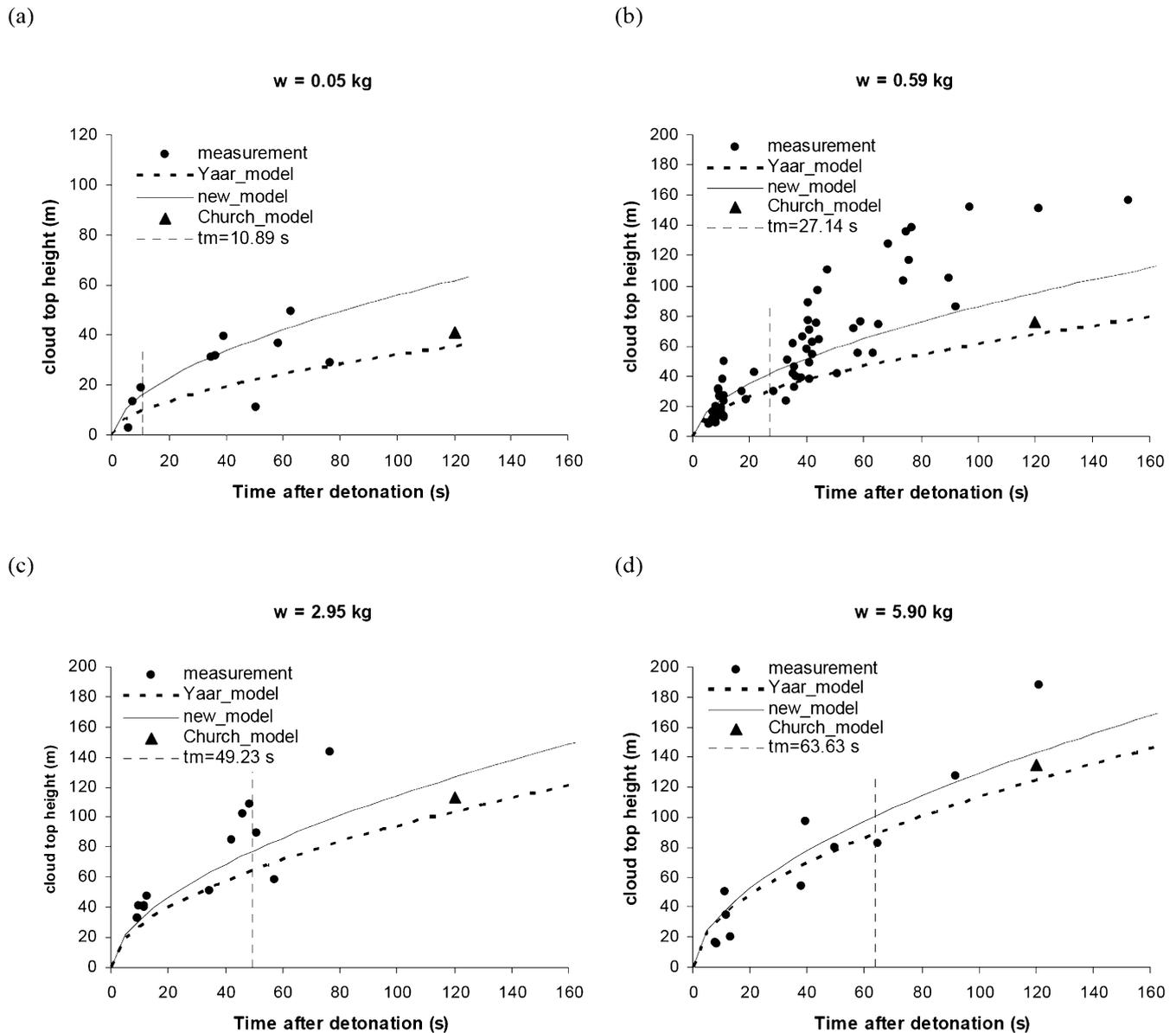
**Figure 5.** Models comparison with field measurement on cloud top height within 2 minutes after detonation of small amount of TNT equivalent (0.05 kg to 5.9 kg). Yaar model means Yaar and Sharon model.
