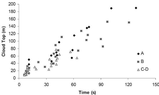
**Figure 4.** Time and atmospheric (Pasquill) stability dependence of the cloud top in the field measurements as result of 0.45 kg C-4 explosive yields.
