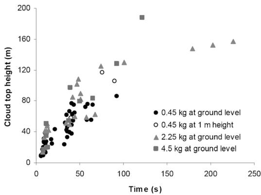
**Figure 3.** Time and charge mass dependence of the cloud top in the field measurements: (a) detasheet less than 0.45 kg; (b) C-4 (0.45–4.5 kg).
