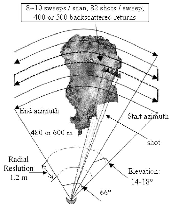
**Figure 1.** Raster scanning pattern of the lidar.
