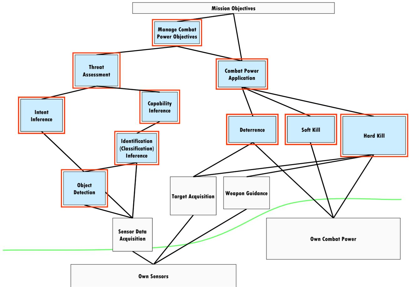
Figure 5: Simplified FAN for the TEWA work domain.
