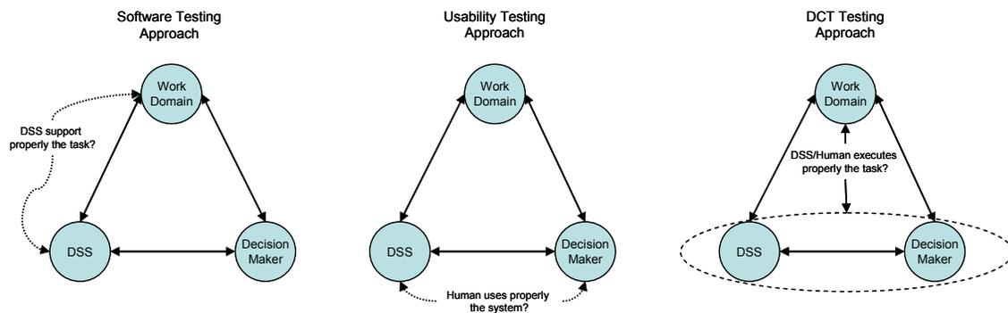
*Figure 1: The focus of Decision Centered Testing (DCT) in relation to more traditional evaluation methods, software testing and usability testing.*
