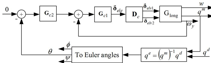
Figure 4. Longitudinal control architecture for hovering mode
