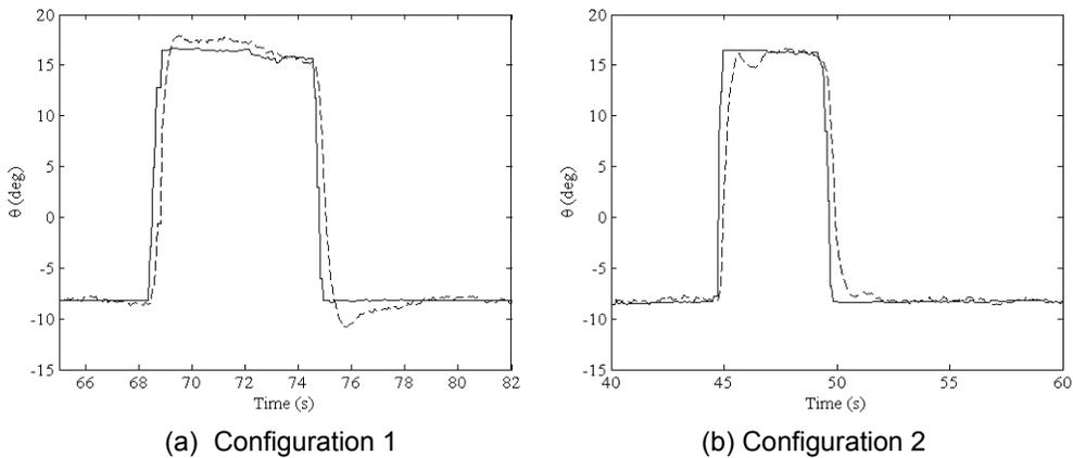
Figure 7. Flight test results magnified: Command ( - ), Response ( - - )
