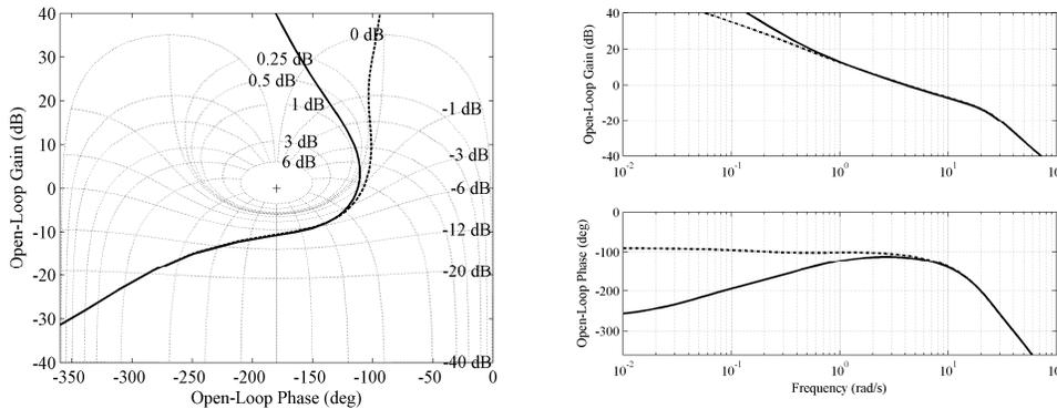
Figure 5. Frequency responses of the external loop: Config. 1 ( - ), Config. 2 ( - - )
