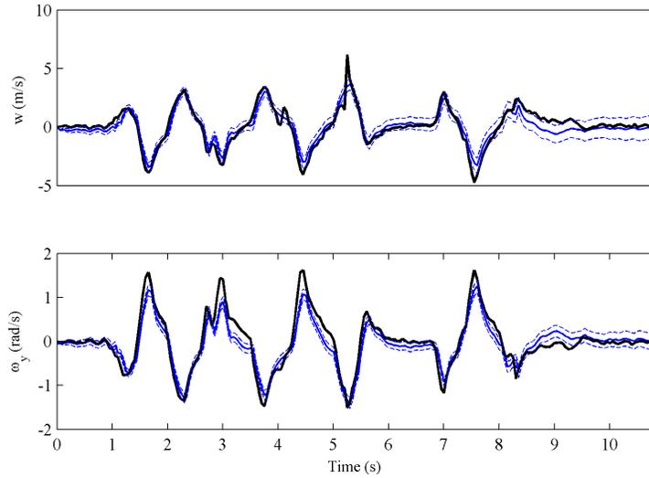
Figure 3. Longitudinal open loop comparison: Measured output (solid black line), Simulated output (solid blue line), Simulated output standard deviation (dashed blue line).
