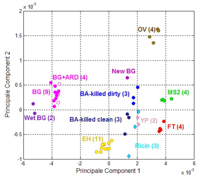
**Figure 2.** Two first components from a Principal Component Analysis (PCA) performed on the simulants LIF signatures.
