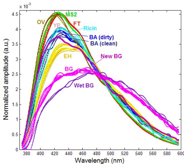
**Figure 1.** LIF signatures of biological agent simulants acquired by SINBAHD during the JBSDS II Tech Demo III trial, DPG, USA, August 2007.
