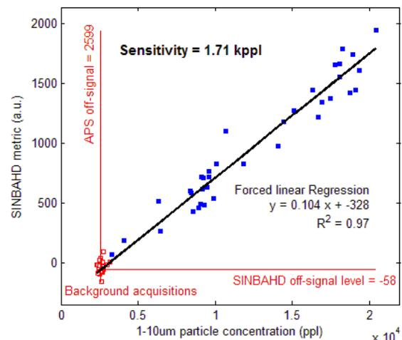
**Figure 4.** Automatic correlation evaluation between SINBAHD and APS data during background (red) and material release (blue) for a 20-m cloud of BG at 1.26 km (T02)
