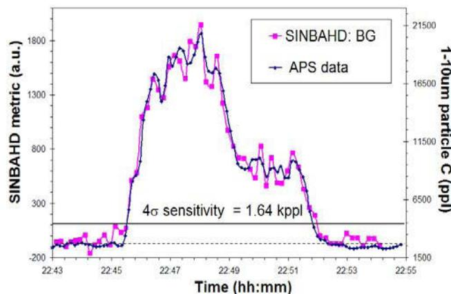
**Figure 3.** SINBAHD metric: BG signature amplitude (pink) and APS data (blue) for release T02 of BG with a 20-m gate at a range of 1.26 km.
