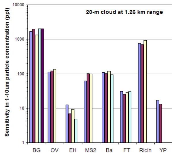
**Figure 6.** SINBAHD sensitivities for various simulants releases obtained in the JABT during the Tech Demo III (20-m cloud at 1.26 km).
