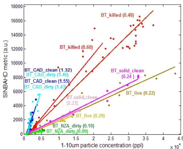
**Figure 5.** Correlation evaluation between SINBAHD metric and APS data for different BT releases (20-m cloud at 1.26 km).
